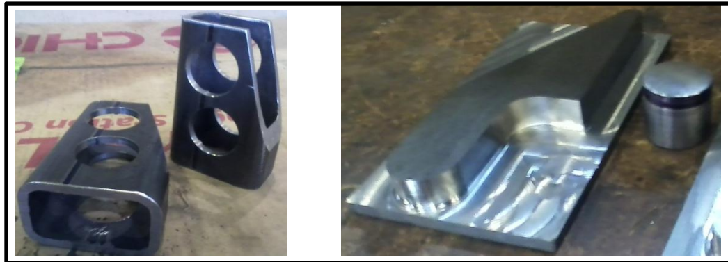
Figure 39: Milling Operations used for the Bucket
