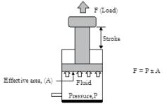
When the pressure (P) is applied to the area (A) of the piston, it develops a force (F).  $-> F = P \times A$
