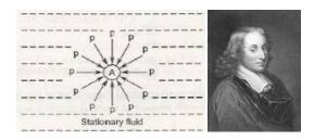
The applications could use fluid as a means to multiply the power. Pascal's law is central to the development of a number of devices, such as hydraulic brakes, hydraulic presses, and hydraulic jacks.
