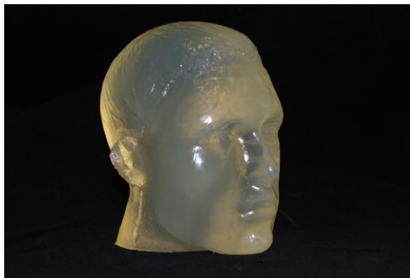
Figure 8 Showing a moulded ballistics gelatine head, picture reference DSCO7286.jpg by Alan McDonald
