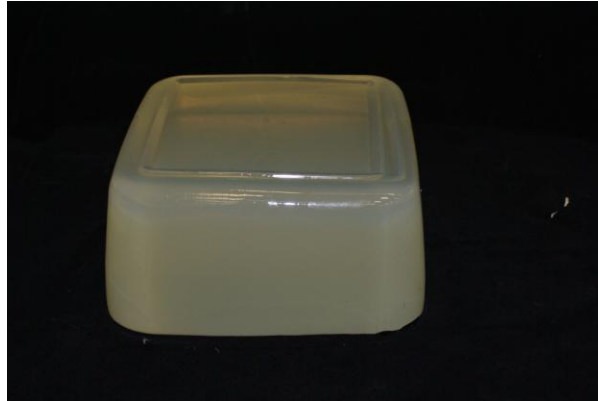
Figure 7 Showing a ballistics gelatine block prior to testing, picture reference DSCO7288.jpg by Alan McDonald.
