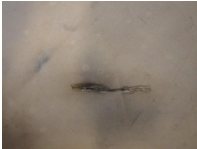
Figure 12 , Showing puncture damage to skin simulant sample, picture reference DSCO1564.jpg, by Alan McDonald.
