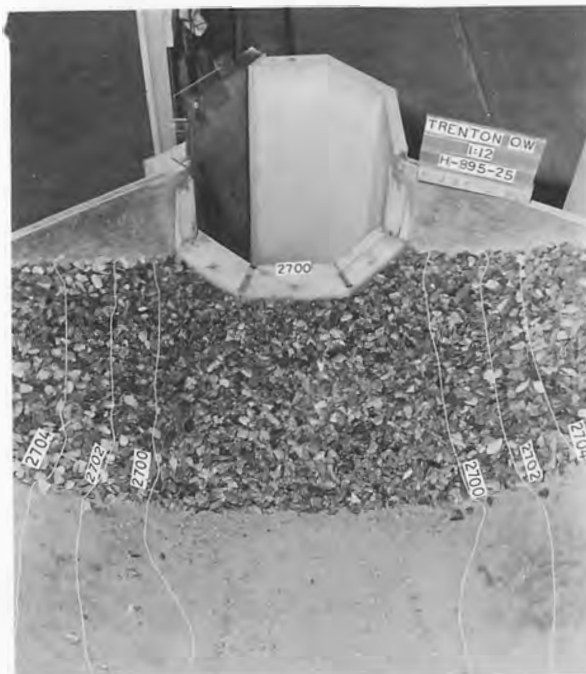
C. Scour after 30 minutes operation at 50% gate opening. Q = 300 cfs. Head at gate, 86.0 feet
