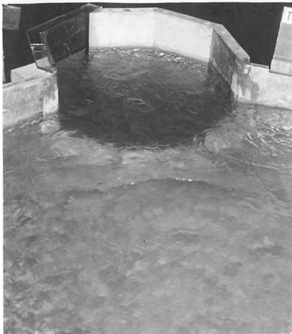
A. Gate 25% Open. Q = 180 cfs. Head at gate = 110.3 feet (Max. reservoir elevation)
