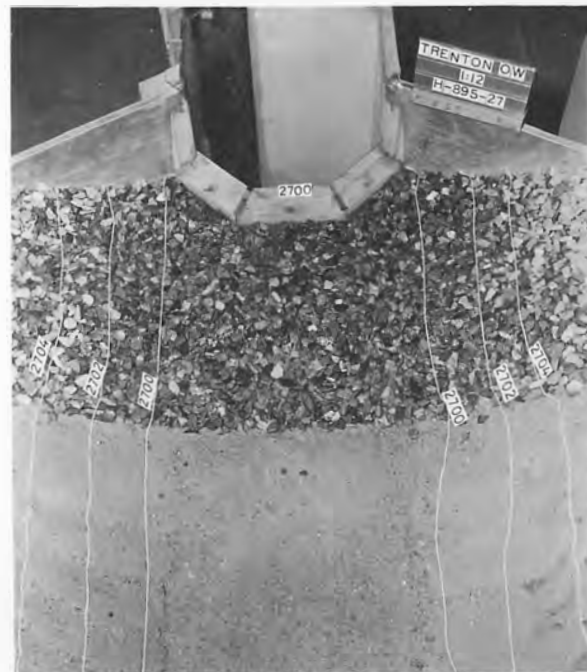
D. Scour after 30 minutes operation at 100% gate opening. Q = 300 cfs. Head at gate, 39.6 feet
