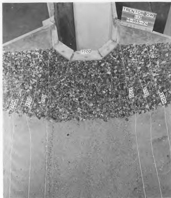
B. Scour after 30 minutes operation at 25% gate opening. Q = 180 cfs. Head at gate = 110.3 feet (Max. reservoir elevation)
