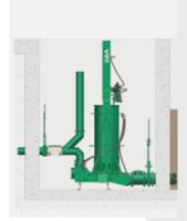
Installation inside a service pit next to the reception pit Provides a flooded inlet to the pump for worry-free operation.
