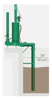
Installation on the floor next to the reception pit Suction pipe 36" (91 cm) from the wall. The pump must be installed in a recess when the reception pit is deeper then 10 feet (3 m).
