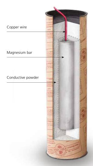
The high purity magnesium bar inside the sacrificial anode will disintegrate slowly and will protect your evacuation line over several years.
