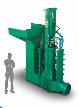
Several types of hoppers are available for installations comprising 1 or 2 barn cleaners, or for skid-steer loader scraped alleys in free stall barns. The pump hopper can be replaced by a suction pipe and reception pit if the manure does not contain bedding.
