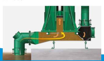
During the evacuation cycle the downstroke of the piston creates sufficient pressure to close the intake valve and open the discharge valve, allowing evacuation of the manure.
