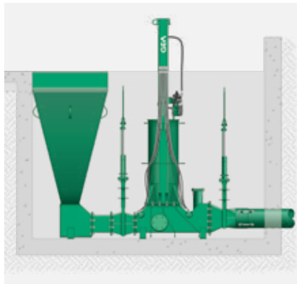
Futuro with manual inlet and outlet guillotines and fitted with a hopper to collect the manure from a cross-gutter cleaner or skid-steer loader
