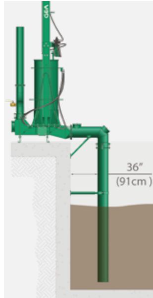
Installation on the floor next to the reception pit Suction pipe 36" (91 cm) from the wall. The pump must be installed in a recess when the reception pit is deeper than 10 feet (3 m).
