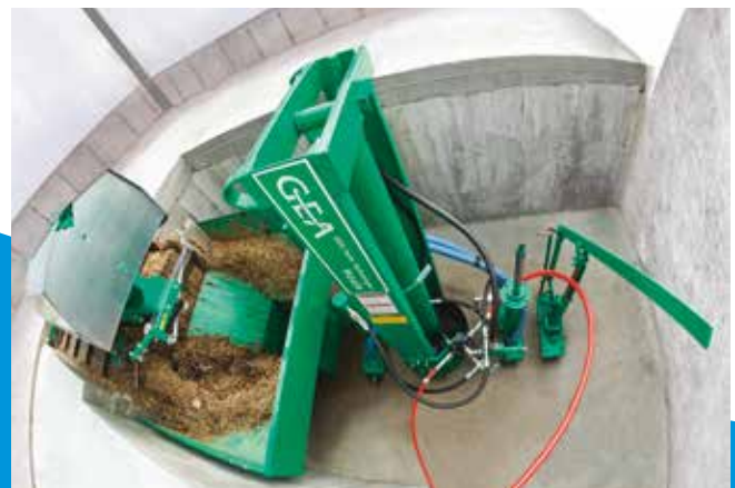
Magnum fed by a 7/8" chain gutter cleaner system and fitted with hydraulic inlet and outlet guillotines and 16" (406 mm) manual safety guillotine.
