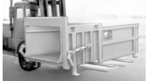
Lifting a compactor from the side
