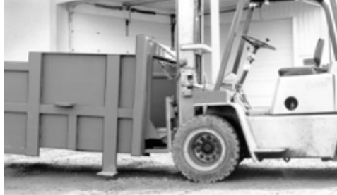
Lifting compactor from the chamber end
