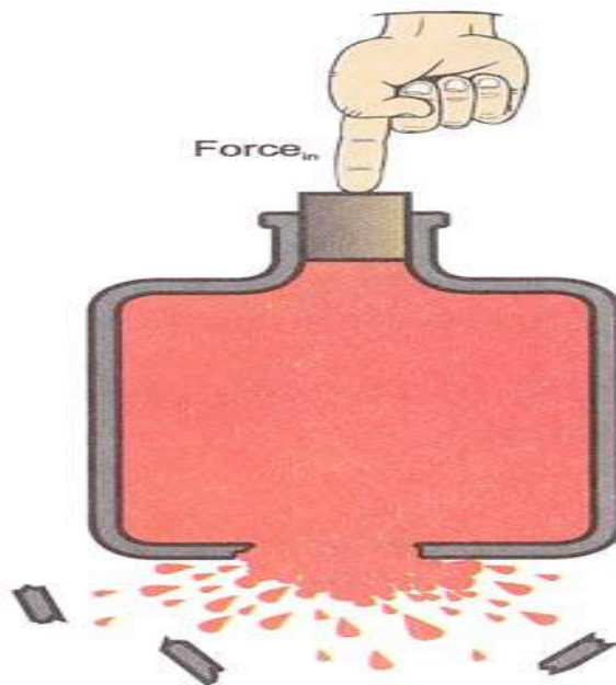
Figure 7 - Container bursting due to pressure
