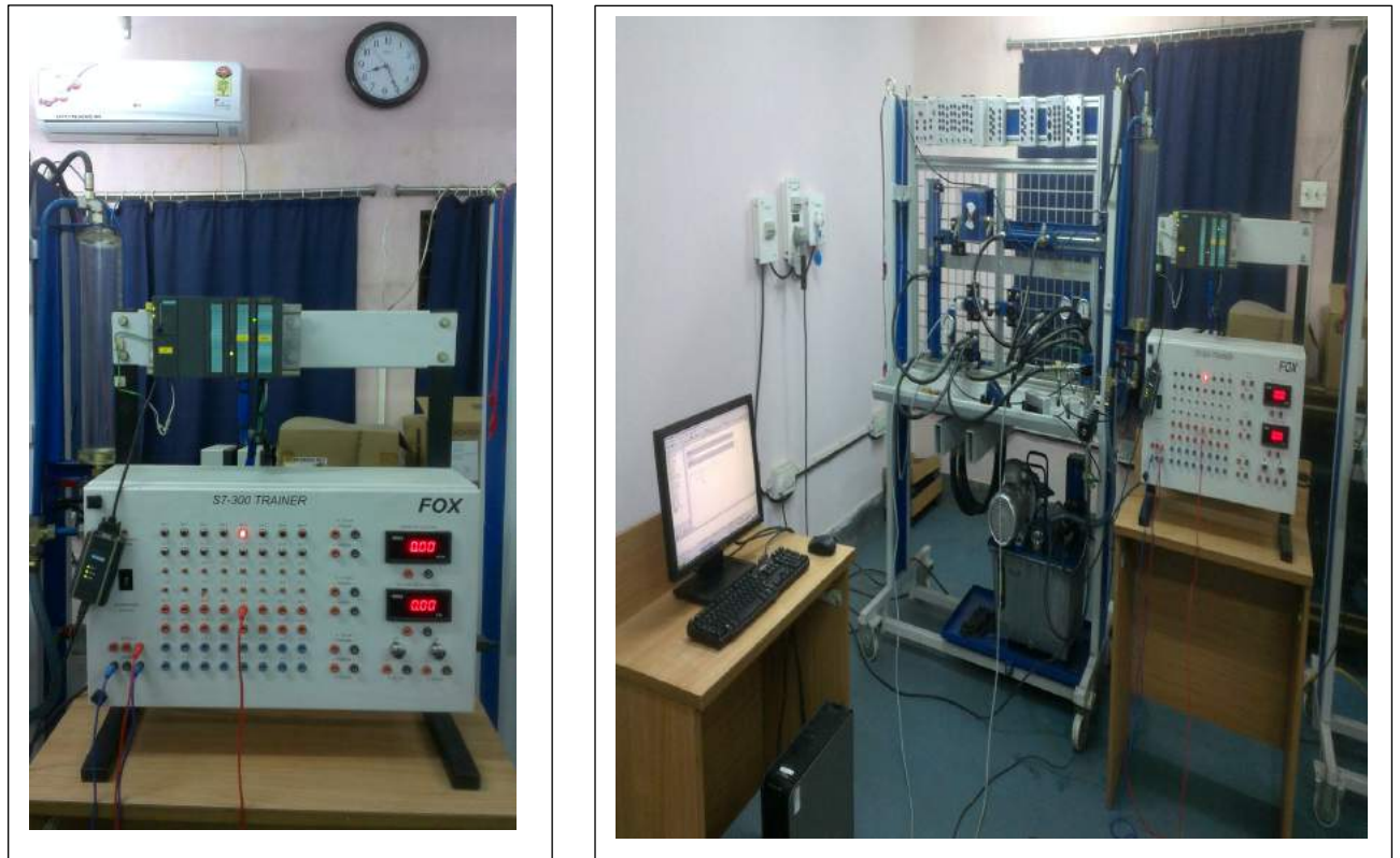
Figure 5 & 6- s7-300 trainer & the total set up.
