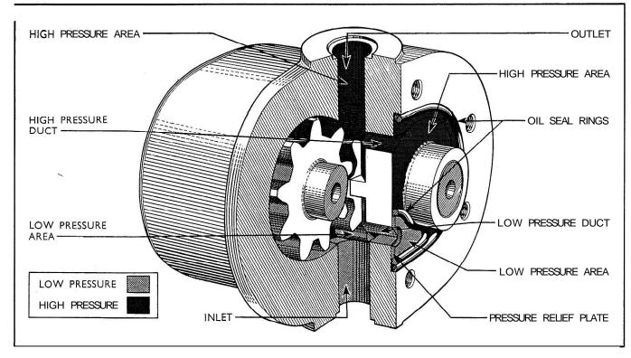
Fig. 181 Sectioned View of Hydraulic Pump
