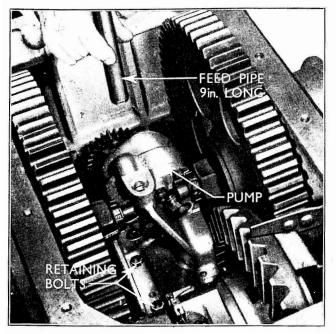
Fig. 193 Removing the Hydraulic Pump Feed Pipe
