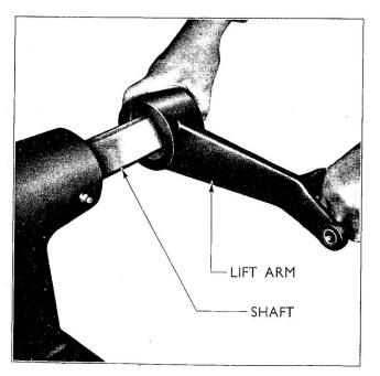
Fig. 195 Fitting a Lift Arm
