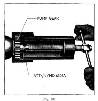
**Removing the Pump Drive Gear**
