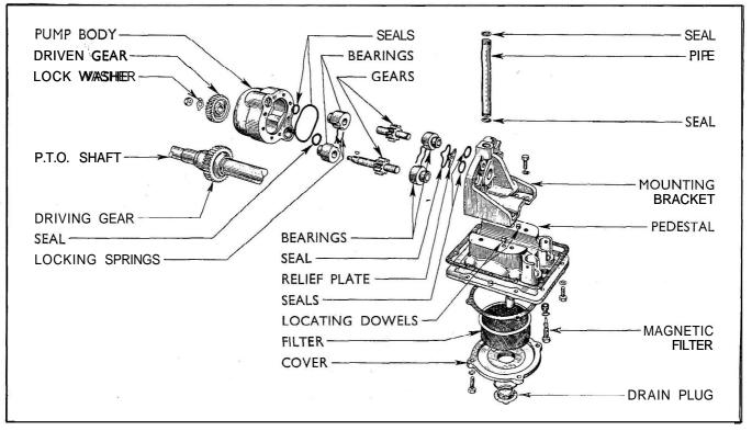
Fig. 199 Exploded View of Hydraulic Pump
