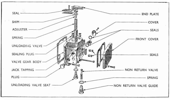
Fig. 194 Exploded View of Valve Control Unit
