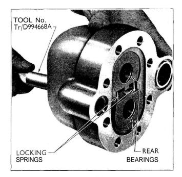
Fig. 203 Removing the Pump Rear Bearings
