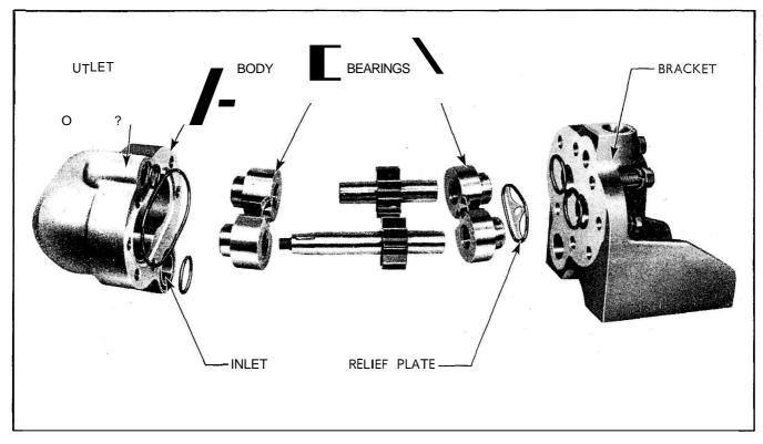
Fig. 200 Exploded View of Hydraulic Pump
