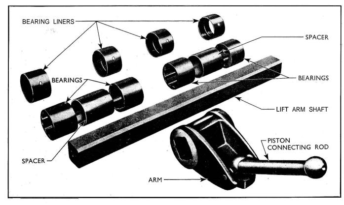
Fig. 198 Exploded View of Lift Arms, Cross-shaft, Bearings and Piston Connecting Rod
