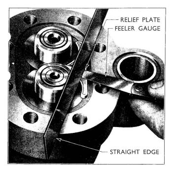
Fig. 204 Checking the Relief Plate Clearance
