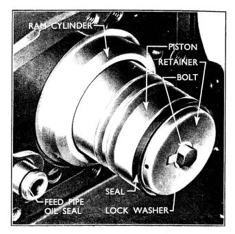
Fig. 196 Fitting the Ram Cylinder Piston
