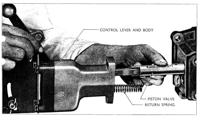
Fig. 191 Fitting the Control Lever and Piston Valve to Body
