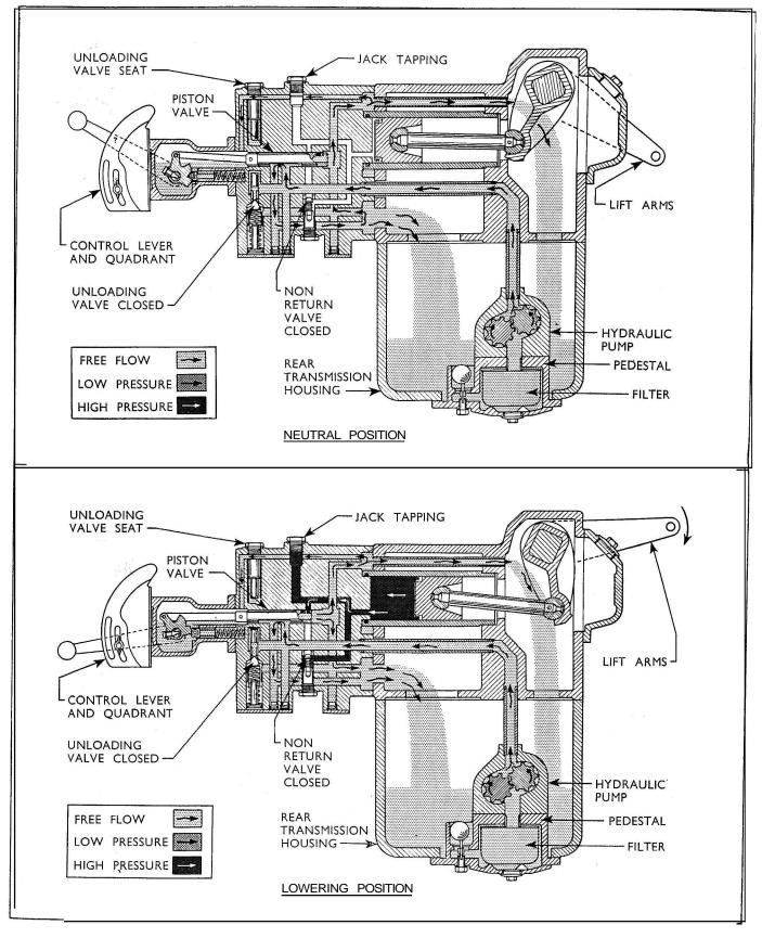
Fig. 183 Diagrammatic Representation of Hydraulic System in Neutral and Lowering Positions
