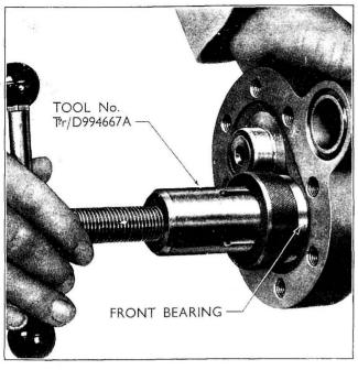
Fig. 202 Removing the Pump Front Bearings
