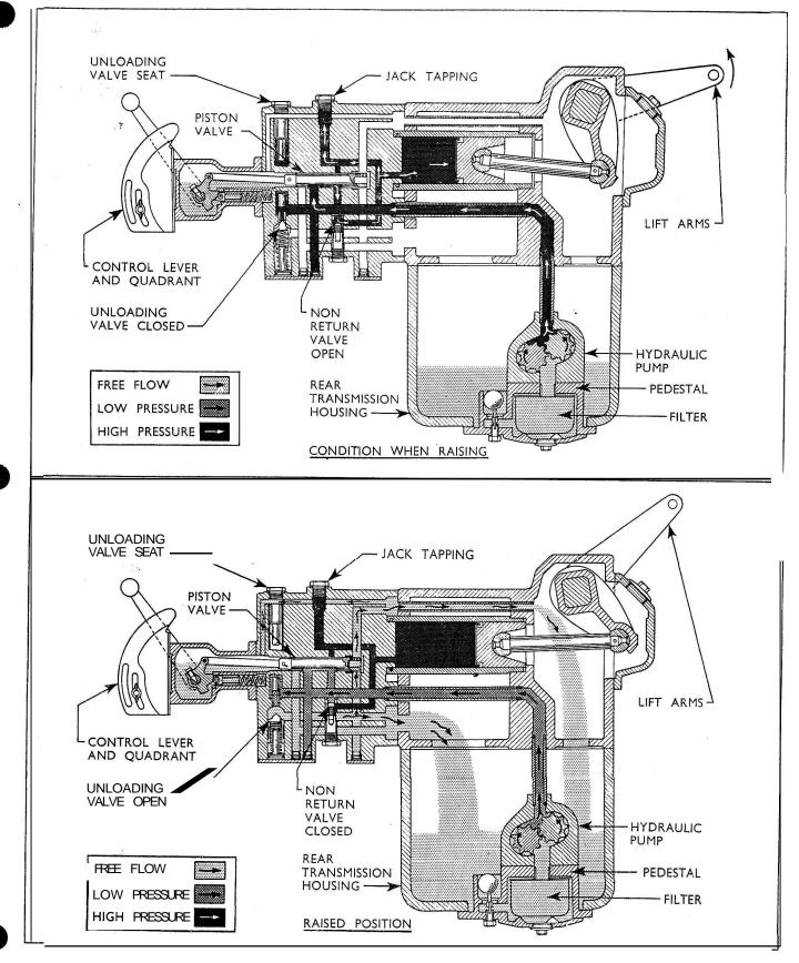
Fig. 184 Diagrammatic Representation of Hydraulic System when Raising and in the Raised Position
