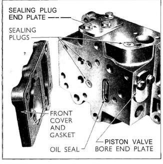
Fig. 189 Valve Body and Cover Plate
