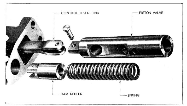
Fig. 183 Piston Valve, Link, Cam Roller and Spring
