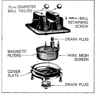
Fig. 180 Exploded View of Early Type Pump Pedestal and Filter
