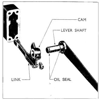
Fig. 192 Fitting the Control Arm
