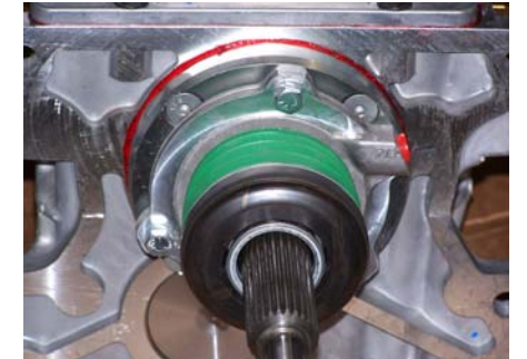
FIG. J CSC PROPERLY INSTALLED
