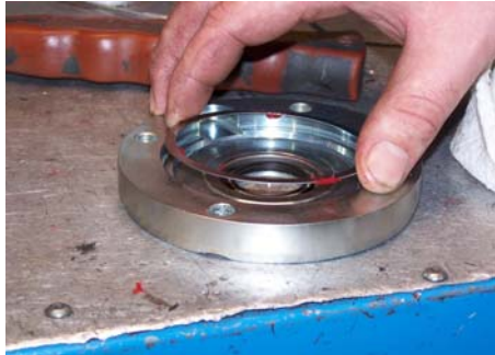
FIG. E (TKO ONLY) INSTALL SHIMS IN RETAINER
