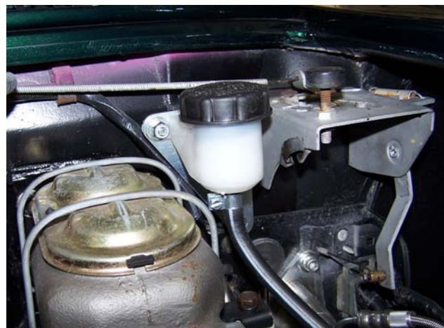
HYDRAULIC RESERVIOR INSTALLED
