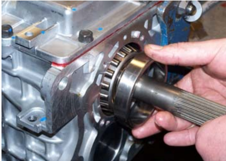
FIG. D (TKO ONLY) INSTALL BEARING RACE IN TRANS
