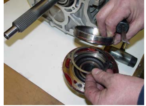
FIG. C (TKO ONLY) REMOVE BRG. RACE AND SHIMS
