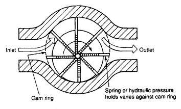
(a) Unbalanced vane pump
