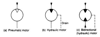
Figure 5.25 Rotary actuator symbols
