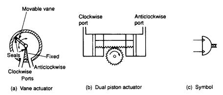
Figure 5.29 Limited motion rotary actuators
