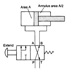
Figure 5.4 Cylinder with equal extend/retract force
