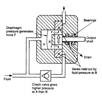
Figure 5.28 Vane operation in hydraulic motor
