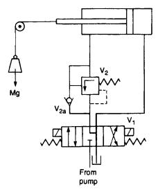
Figure 5.42 Counterbalance circuit
