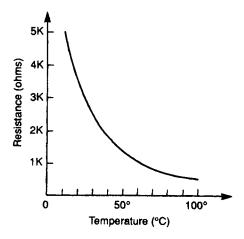
**Figure 1.22** Typical resistance temperature curve for NTC thermistor
