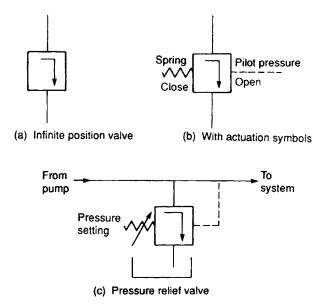
Figure 4.8 Infinite position valve symbols
