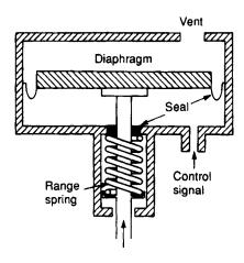
Figure 7.19 Fail-down actuator
