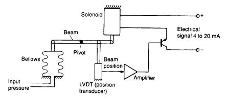
Figure 7.26 Pressure to current (P–I) converter
