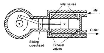
Figure 3.4 Double-acting compressor
