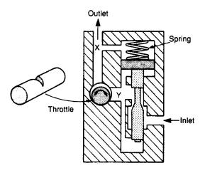
Figure 5.34 Pressure compensated flow control valve
