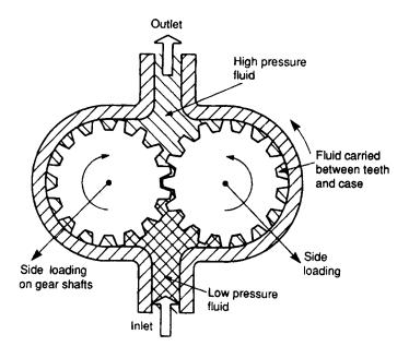
Figure 2.7 Gear pump
