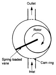
Figure 3.9 Vane compressor
