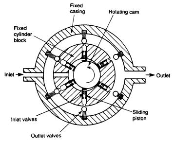
Figure 2.12 Radial piston pump
