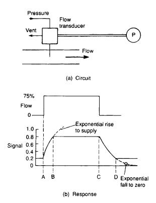
Figure 7.2 Advantage of an offset zero
