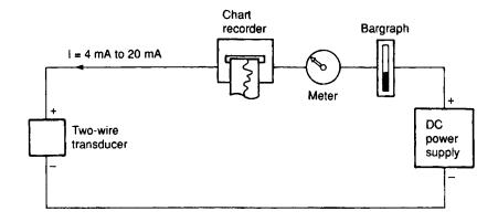
Figure 1.15 Advantages of two-wire transducers
