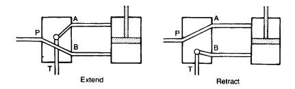
Figure 4.2 Internal valve operation
