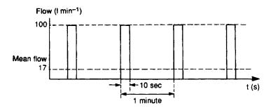
**Figure 6.2** A simple system with uneven demands. To supply this without an accumulator a 100 l min<sup>-1</sup> is required although the mean flow is only 17 1/min
