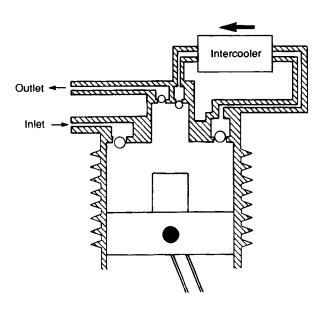
Figure 3.6 Combined two-stage compressor
