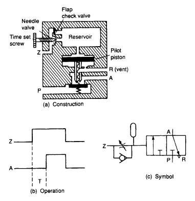
Figure 4.28 Pneumatic time delay valve
