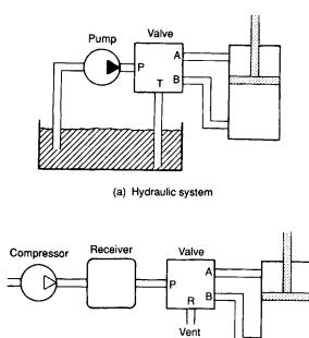
Figure 4.1 Valves in a pneumatic and hydraulic system
