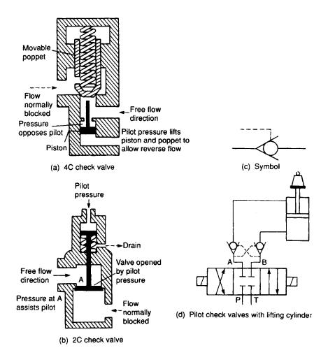
Figure 4.23 Pilot-operated check valves
