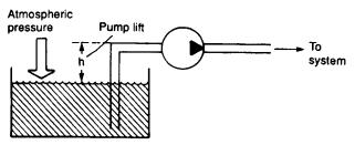
Figure 2.4 Pump lift
