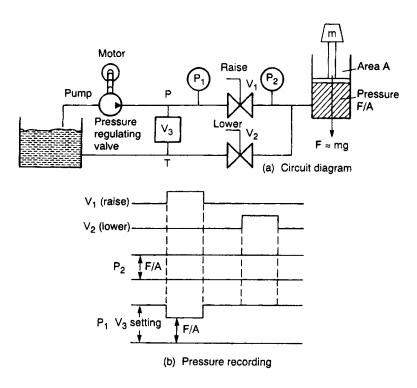
Figure 2.5 Action of pressure regulation
