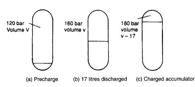
Figure 6.5 Sizing an accumulator
