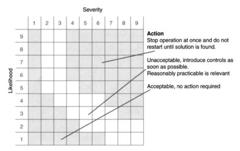
Figure 8.1 A typical risk assessment table. Although this is based on a real application, it should not be applied elsewhere without supporting study and documentation. The main point of a risk assessment is identifying and reducing the risks associated with a specific task
