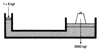
Figure 1.10 Mechanical advantage
