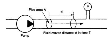
Figure 2.3 Derivation of pump power
