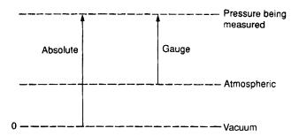
Figure 1.7 Relationship between absolute and gauge pressures
