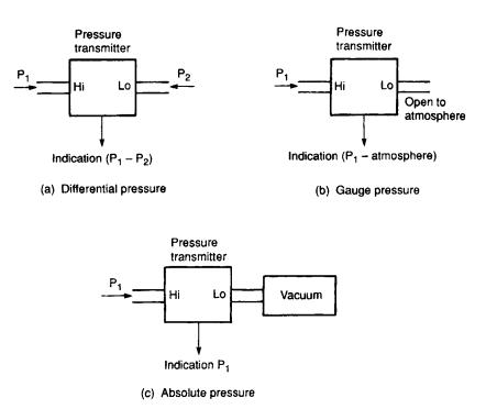
Figure 1.6 Different forms of pressure measurement
