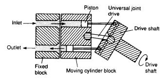
Figure 2.15 Bent axis pump
