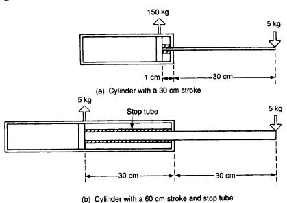
Figure 5.11 Side loads and the stop tube
