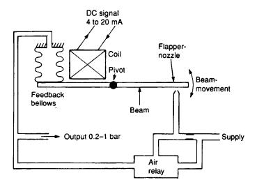
Figure 7.25 Current to pressure (I–P) converter
