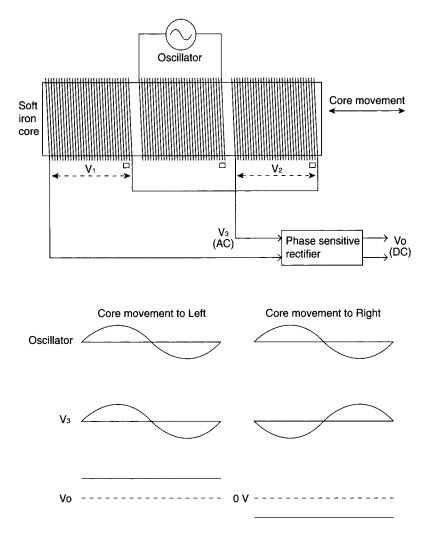
The use of an LVDT to give position control of the valve spool. The LVDT can be connected to the pilot or main spool. (a) The circuit arrangement of the LVDT and phase sensitive rectifier. (b) Output signals for core displacement to left and right
