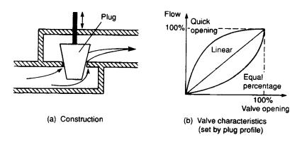
Figure 7.12 The plug valve
