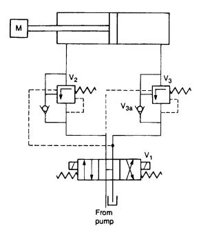
Figure 5.43 Braking a high inertia load
