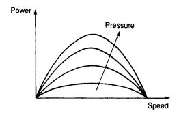
Figure 5.24 Power/speed curve for pneumatic rotary actuator
