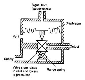
Figure 7.5 The air relay
