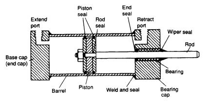
Figure 5.8 Construction of a typical cylinder
