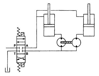
Figure 5.39 Cylinder synchronisation with linked hydraulic motors
