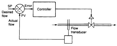
Figure 7.1 Closed loop control
