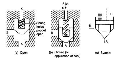
Figure 4.46 Cartridge logic valve
