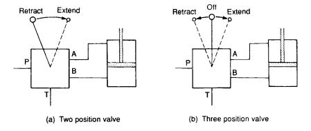
Figure 4.3 Valve control positions
