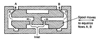
Figure 5.38 Flow divider valve
