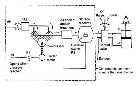
Figure 1.3 Pneumatic solution
