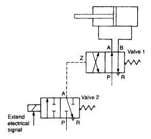
Figure 4.16 Pilot-operated valve
