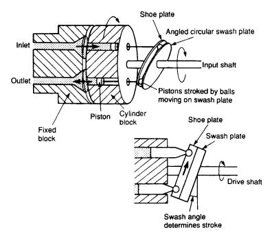
Figure 2.14 Axial pump with swash plate
