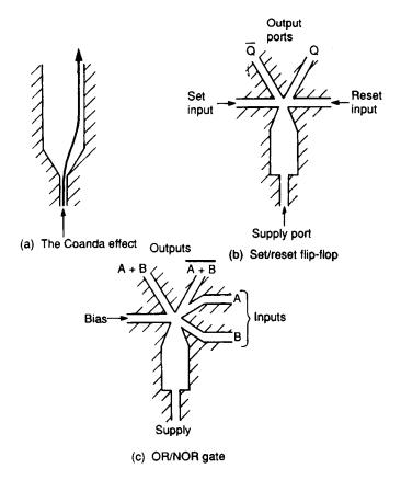
Figure 7.32 Fluidic logic
