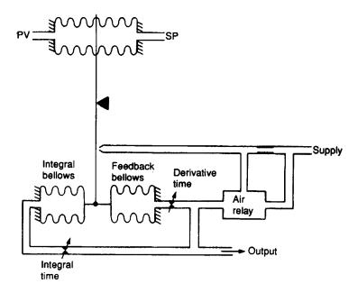
**Figure 7.9** Three term (P + I + D) controller
