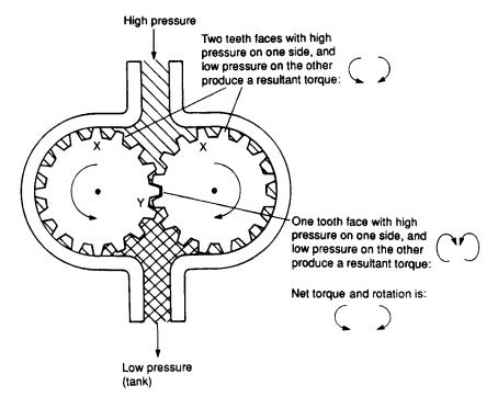
Figure 5.26 A gear motor
