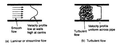
Figure 1.16 Types of fluid flow
