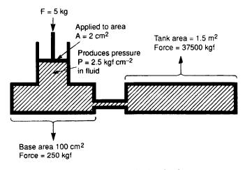
(a) Forces and pressure in closed tanks
