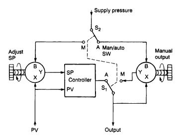
Figure 7.11 Internal arrangement giving bumpless transfer
