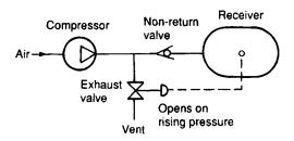
Figure 3.15 Receiver pressure control using compressor outlet valve
