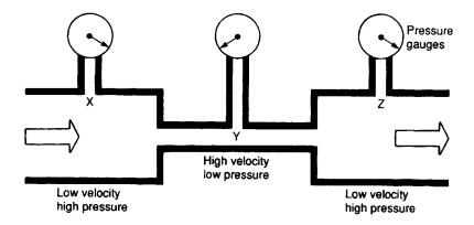
Figure 1.17 Relationship between flow and pressure
