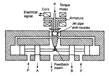
Figure 4.41 Jet pipe servo valve
