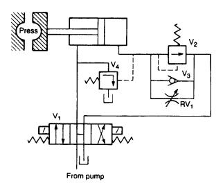
Figure 5.47 Controlled decompression circuit
