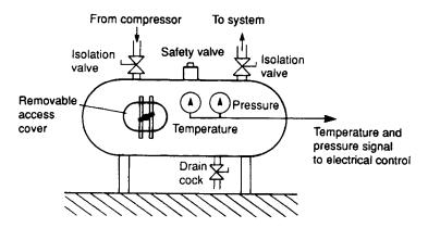
Figure 3.13 Compressed air receiver
