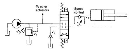
Figure 5.31 Meter in speed control
