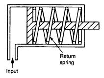
Figure 5.5 Single-acting cylinder
