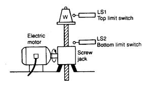
Figure 1.1 Electrical solution, based on three phase motor
