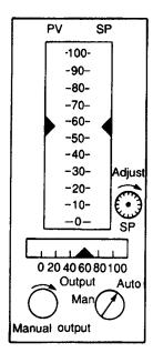
Figure 7.10 Front panel of a typical controller
