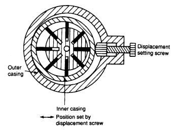
Figure 2.11 Variable displacement vane pump
