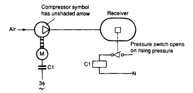
Figure 3.14 Receiver pressure control via motor start/stop
