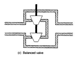
Figure 7.15 Dynamic forces acting on a valve
