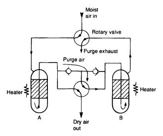
Figure 3.22 Adsorption dryer
