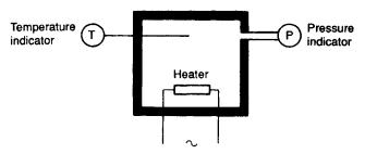
Figure 1.25 Relationship between temperature and pressure
