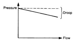
Figure 3.28 Response of simple pressure regulators
