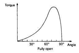
Figure 7.16 Torque on a butterfly valve
