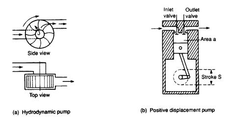
Figure 2.2 Types of hydraulic pump
