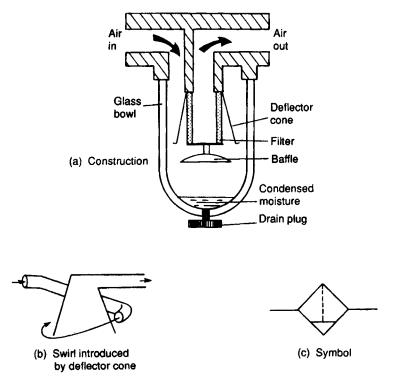
Figure 3.19 Air filter and water trap
