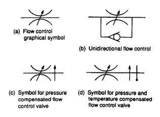
Figure 5.35 Flow control valves
