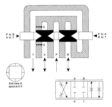
Construction and symbol for a proportional valve. Figure 4.30 When used with a cylinder with 2:1 full bore to annulus area ratio, half the V cutouts will be provided on one of the P lands
