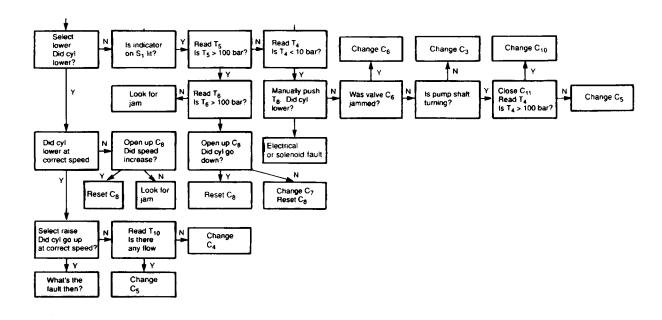
Figure 8.11 Fault-finding flowchart for circuit of Figure 8.10
