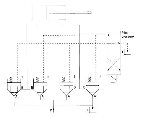
**Figure 4.48** Direction control using four cartridge valves. As shown the cyclinder will fully extend or fully retract. If two solenoid valves are used, one for open, one for close, the cylinder can hold position
