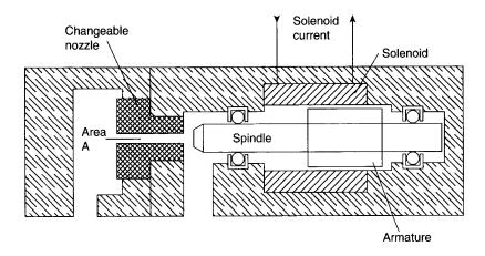
**Figure 4.39** Proportional pressure control valve. The pressure is given by the force produced by the solenoid divided by the area
