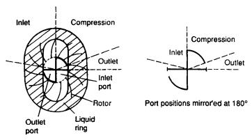
Figure 3.10 Liquid ring compressor
