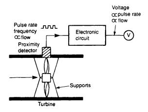
Figure 1.19 Turbine flowmeter
