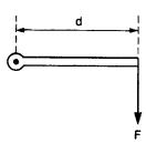
Figure 1.8 Definition of torque
