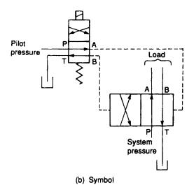
Figure 4.18 Pilot-operated valve
