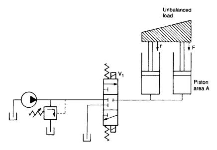
Figure 5.37 Linked cylinders with unbalanced load
