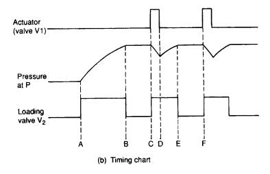
Figure 6.3 System with an accumulator
