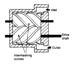
Figure 3.8 Dry screw rotary compressor
