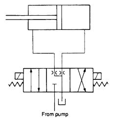
Figure 5.46 Valve with central damping block
