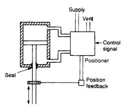
Figure 7.20 Double-acting cylinder (holds position on failure)
