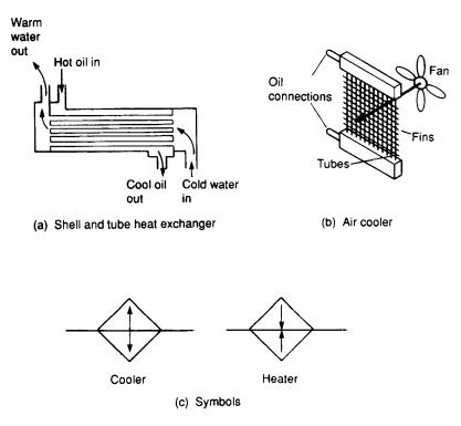
Figure 6.7 Coolers and heat exchangers
