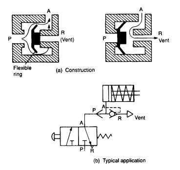
Figure 4.26 Fast exhaust valve
