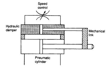
Figure 5.36 Speed control of pneumatic cylinder
