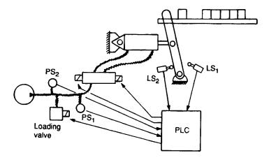
Figure 8.8 A typical sequencing application
