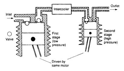
Figure 3.5 Two-stage compressor
