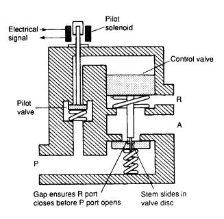
Figure 4.17 Construction of a pilot-operated 3/2 valve
