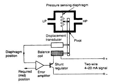
Figure 1.14 Force balance pressure transducer
