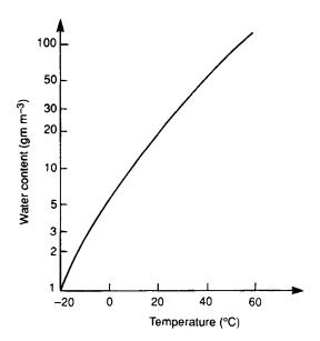
Figure 3. 17 Moisture content curve
