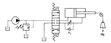
Figure 5.32 Meter out speed control for overhauling load
