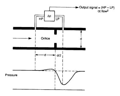
Figure 1.20 Orifice plate flowmeter
