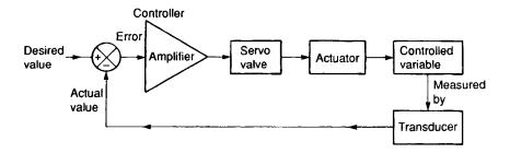
Figure 4.43 A feedback control system
