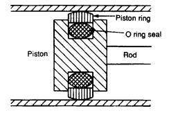
Combined piston ring and O ring seal (not to scale) Figure 5.21
