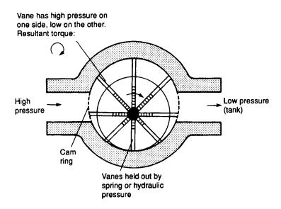
Figure 5.27 A vane motor
