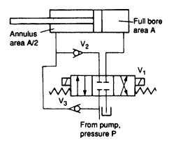
Figure 5.41 Regeneration circuit
