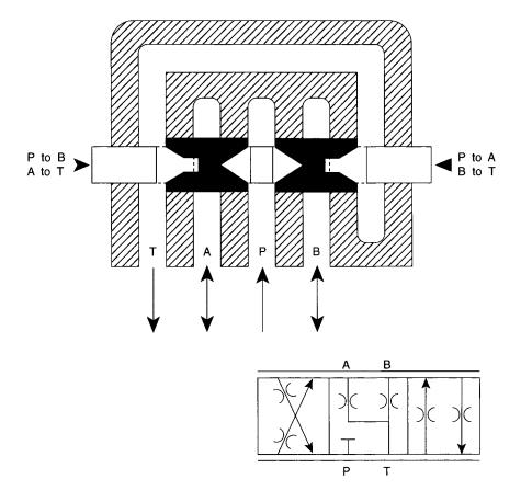
**Figure 4.31** Construction and symbol for a proportional valve with A and B ports linked to tank in the null position
