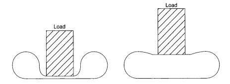
**Figure 5.48** The use of pneumatic bellows gives a simple way of raising and lowering a load
