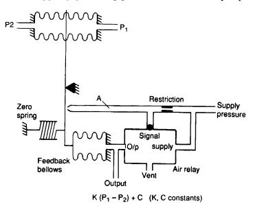
Figure 7.6 The force balance principle
