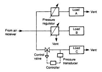
Figure 3.24 Three types of pressure regulator
