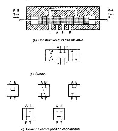
Figure 4.14 Three position four-way valves
