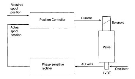
**Figure 4.33** Position of the spool in a proportional valve with an LVDT and a phase sensitive rectifier. In many systems the oscillator, LVDT and phase sensitive rectifier are now included in the valve itself
