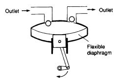
Figure 3.7 Diaphragm compressor, used where air must not be contaminated
