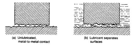
Figure 6.8 Need for lubrication from hydraulic fluid
