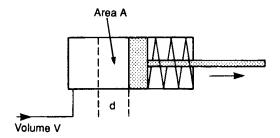
Figure 5.7 Derivation of cylinder speed
