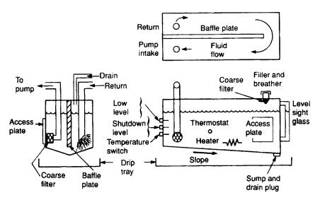
Figure 6.1 Construction of a hydraulic reservoir
