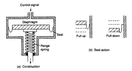
Figure 7.18 Fail-up actuator
