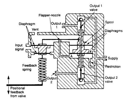
Figure 7.22 Force balance valve positioner
