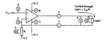
Figure 8.2 Test measurement points on an electronic circuit
