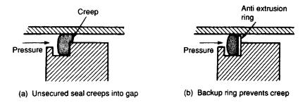
Figure 5.20 Anti-extrusion ring
