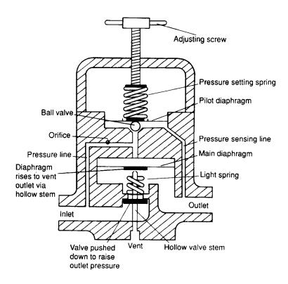
Figure 3.29 Pilot-operated regulator
