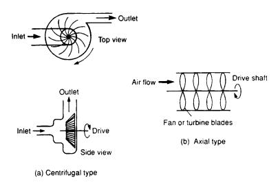
Figure 3.12 Non-positive displacement compressors (Blowers)
