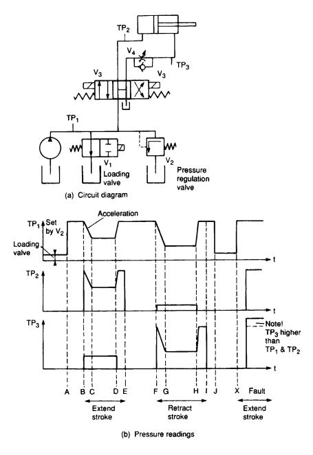
Figure 8.7 Fault-finding with pressure test points
