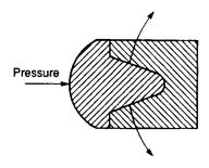
Figure 5.19 The composite seal
