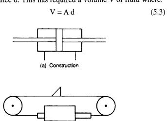
Figure 5.6 Double rod cylinder (with equal extend/retract force)
