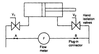
Figure 8.4 Checking flow available at an actuator
