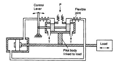
Figure 4.44 Power assistance using mechanical servo valve
