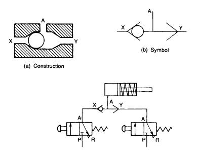
Figure 4.25 Pneumatic shuttle valve
