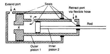
Figure 5.12 Two-stage telescopic piston
