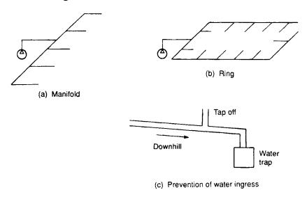
Figure 6.11 Pneumatic piping
