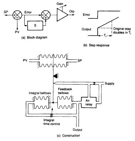
Figure 7.8 Proportional plus integral (P + I) controller
