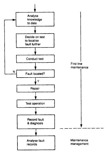
Figure 8.5 Fault-finding process
