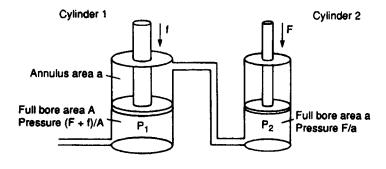
Figure 5.40 Cylinder synchronisation with series connection
