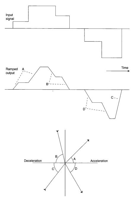
**Figure 4.37** Ramped response. Four quadrant operation is shown, single ramp rate and two quadrant operation are more common. (a) Effect of applying ramps with four quadrant feature. (b) Definition of the four quadrants
