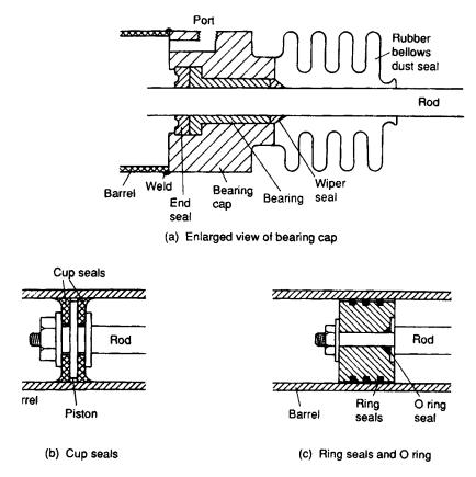
Figure 5.9 Cylinder constructional details
