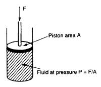
Figure 1.4 Pressure in a fluid subjected to a force
