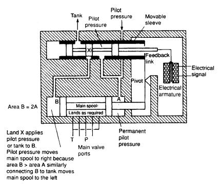
Figure 4.40 Two-stage servo valve
