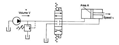
Figure 5.30 Speed control by pump volume
