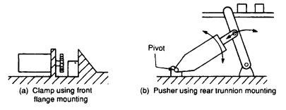
Figure 5.14 Basic mounting types
