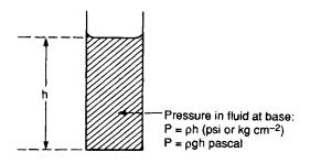
Figure 1.5 Head pressure in a fluid
