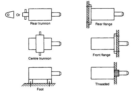
Figure 5.15 Methods of cylinder mounting
