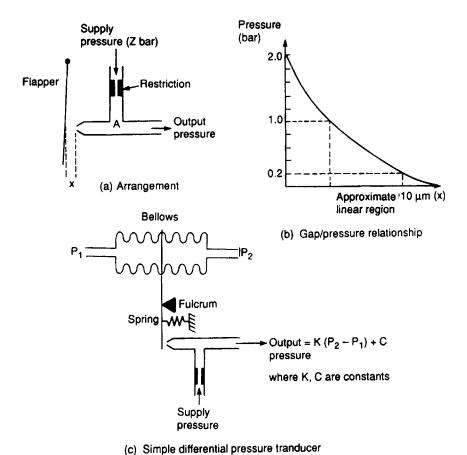
Figure 7.3 The flapper-nozzle, the basis of pneumatic process control
