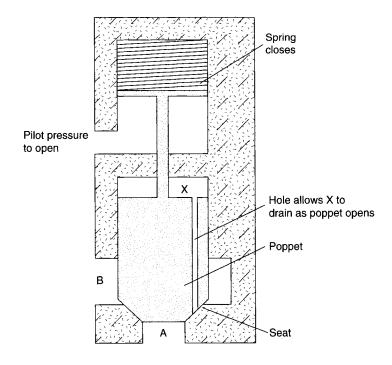
Figure 4.47 Normally closed, pilot to open, cartridge valve
