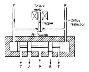
Figure 4.42 Flapper jet servo valve
