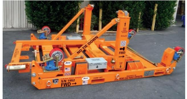
unit, with engine. Tow bar stows on base frame when not in use. Maximum towing speed of unit is 5 km/h (3 MPH). Built-in shock absorbing mounts cushion all transport movements. A series of Tie-down rings (14) offer secure retainment during long distant hauling of unit.
