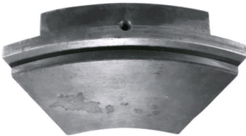
Tin oxide damage of thrust shoe.
