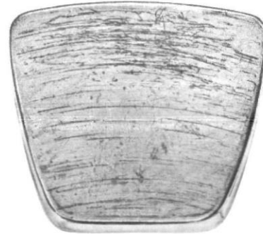
Scoring due to foreign matter or “dirt”
