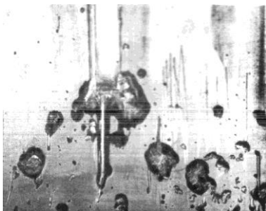
Pitting due to foreign matter or “dirt”
