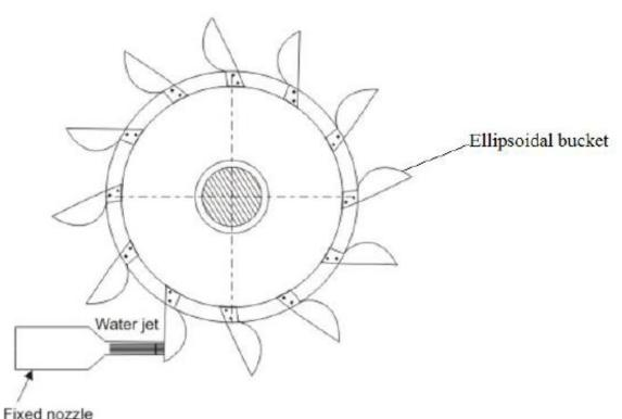
$V_{Water-jet} = C_V[2gH]^{1/2} \, m/s$
