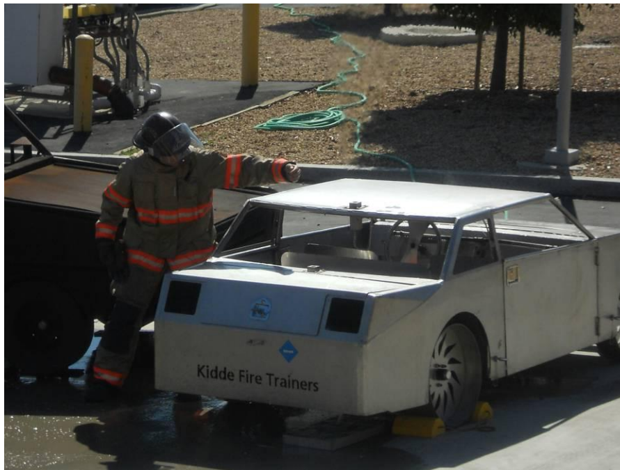
Figure 1. FCV burn prop fabricated by Kidde Fire Trainers. A nearly invisible hydrogen flame is burning from the top of the FCV. Here the instructor is demonstrating the relative lack of radiant heat from a hydrogen flame compared to other flammable gases such as propane.
