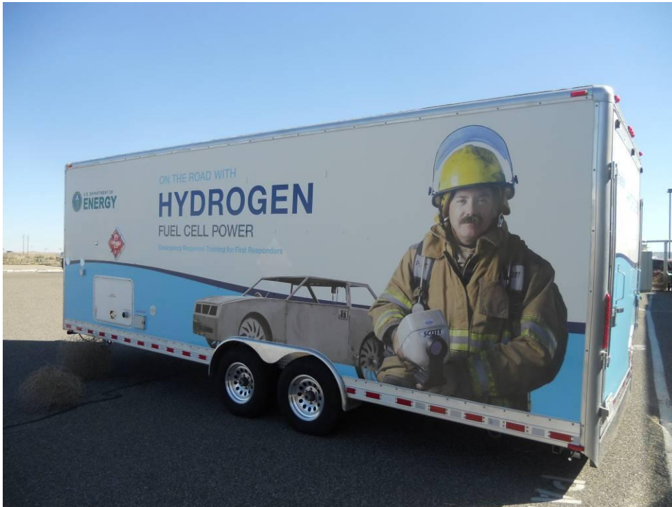
Figure 4. The burn prop is transported to training facilities in this trailer that also contains hydrogen, compressed air, and propane used in the live-fire training exercises.
