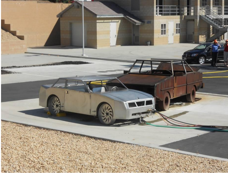
Figure 5. Hydrogen FCV burn prop (left) staged with OCFA propane-fueled burn prop for live-fire training/demonstration.
