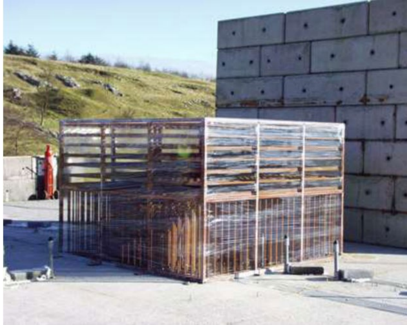
Figure 14: Congestion region or grid where gas was filled then ignited (from [47])
