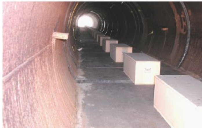
Figure 5: Model of Vehicles in Tunnel (from [40])
