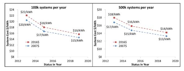
Figure 4. Comparison of storage system cost status in 2007\$ and 2016\$ as reported in 2013 [13], 2015 [14], and in 2019. Costs are for annual productions of 100,000 units (left) and 500,000 units (right).
