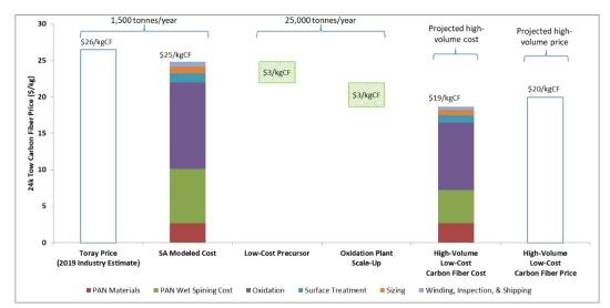
Figure 2. Comparison of current T700S *prices* with projected high-volume carbon fiber (CF) *prices*. The ratio of modeled carbon fiber *cost* at low (1,500 tonnes per year) and high (25,000 tonnes per year) volume are used to scale the quoted low-volume T700S to a projected high-volume carbon fiber *price* assuming processing *cost* savings from the low-cost precursor and oxidation plant are realized. PAN – polyacrylonitrile
