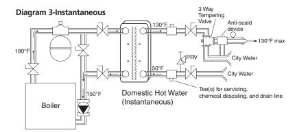
**Piping:** Tee(s) on the output side of the HX are recommended for convenience in event that future chemical descaling and cleaning is required.
