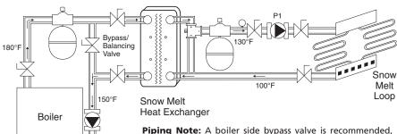
**Piping Note:** A boiler side bypass valve is recommended, but not required. A 3-Way Tempering valve or motorized control valve on the snow melt side is required.
