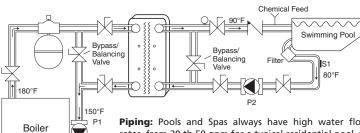
**Piping:** Pools and Spas always have high water flow rates, from 30 th 50 gpm for a typical residential pool, to higher gpms for commercial applications. Because the MPN Series is a high efficiency heat exchanger and does not require the full pool gpm flow, a BYPASS balancing valve is required to bypass 50% to 80% of the pool water. This bypass/balancing valve should be adjusted and permanently set at start-up.
