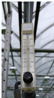
Figure 16. Model: H-03216-04: 65 mm variable area aluminum flow meter with valve and glass float for O 2 . Manufacturer: Cole Parmer Instrument Co., Niles, IL
