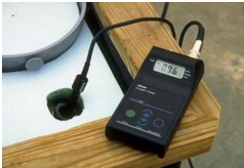
Figure 18. Dissolved oxygen sensor. DO levels should be greater than 4 ppm to prevent growth inhibition. Visible signs of stress may be observed at 3 ppm.
