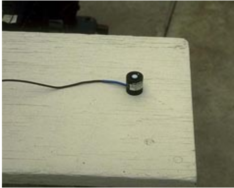
Figure 17. Quantum PAR sensor to measure light available for photosynthesis. Foot-candle sensor and lux meters are inappropriate because they are designed to quantify the sensitivity of the human eye and overestimate (~25%) the light available for photosynthesis
