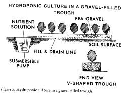
The plumbing-system lines and submersible pumps should have the capacity to fill the beds in about 15 minutes, and allow complete drainage in 30 to 45 minutes.
