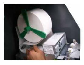
5) Insert the leading edge of paper into the loading guide of the receipt printer slowly. When the machine is initialized, the paper is going to start feeding
