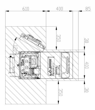
Fig. 4.1 Installation space #1 (Plane view)
