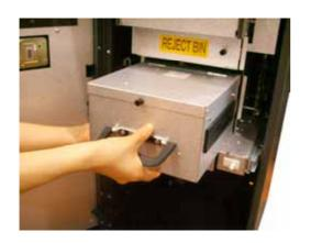
7) With one hand holding the cash cassette handle and the other hand supporting the cash cassette from the bottom, place the cash cassette carefully on the set guide of the Cash Dispensing Unit and push it in until it is locked in place.
