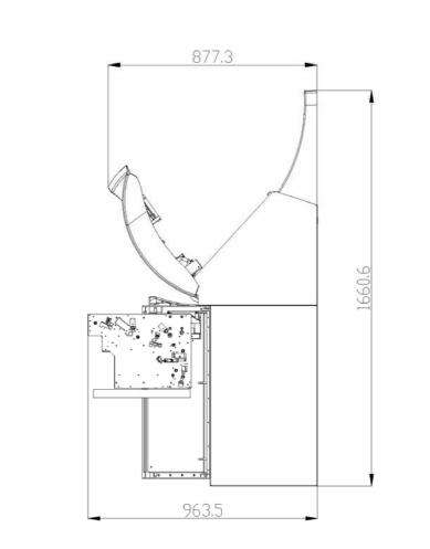
Fig. 4.2 Installation space #2 (Side view)
