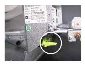
3) After finishing clearing the receipt, load the receipt paper properly. Please make sure to return the green lever to its right place one more time before closing the Front Panel. When finished loading paper, close the Front Panel and remove the key.
