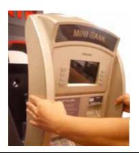
7) When finished loading paper, close the Front Panel and remove the key.
