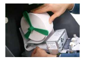
4) The shiny side of the paper should be faced up to be printed properly and the metallic tension guide should be surrounded with paper to reduce the tension during feeding
