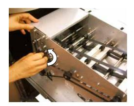
2) Turn the pulley located in left upper in order to move jammed note into a well removed position
