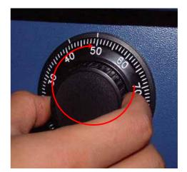
Note: The center scale mark is used to open the safe unit
