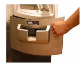
1) Turn the Security Cover key clockwise to open the Security Cover.
