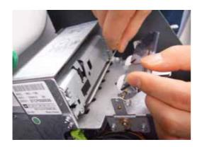
2) To take out a jammed paper in front of transport path, lift up the transparent window guide and remove the jamming receipt carefully.
