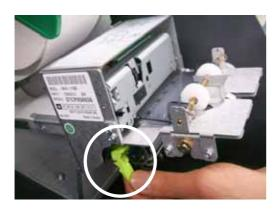
Open the Front Panel with key and pull this outward completely with hands. To remove a jammed paper inside transport path, press the green lever down to release the lower roller assembly.
