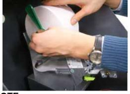
3) Remove the green paper holder by carefully pulling it off and add the receipt paper into the spindle. And then insert the green paper holder tightly again to fix it.
