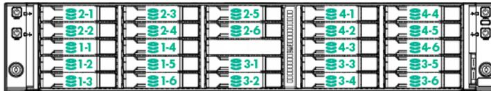
**Figure 1: Disk drive numbering (four-node system)**
