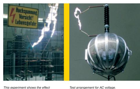
Test arrangement for AC voltage.
