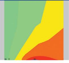
Figure 9: Electric potential at a semiconductive corona protection of the stator end winding.
