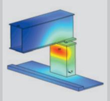
Figure 5: Power loss density in circuit rings and flux lines in surrounding air.
