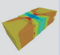
Figure 10: Nonlinear stress-strain analysis of a periodic segment of a rotor rim for homogenized FE analysis.
