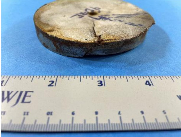
Figure 31. Core in the bottom flange plate at the arrested crack tip.
