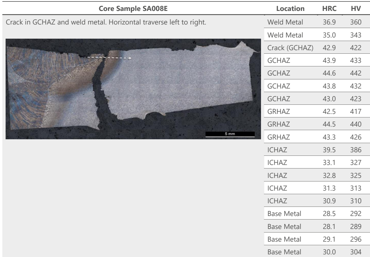
Figure 48. Microhardness traverse for Core Sample SA008E.
