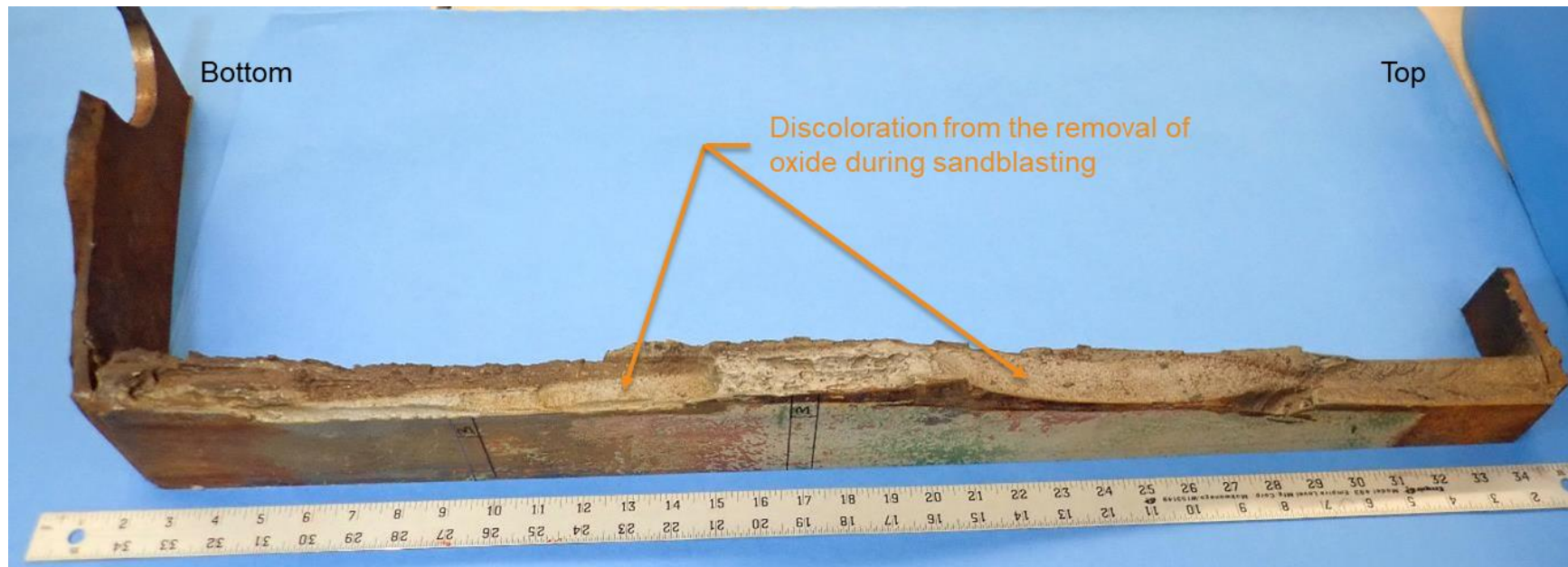
Figure 19. West fracture surface (left piece shown in Figure 17).
