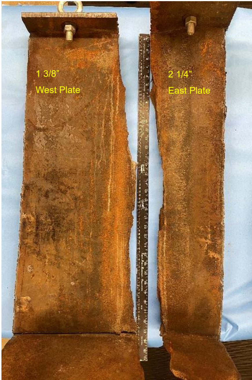
Figure 17. As-received sample from the fracture at NB222W for laboratory analysis.
