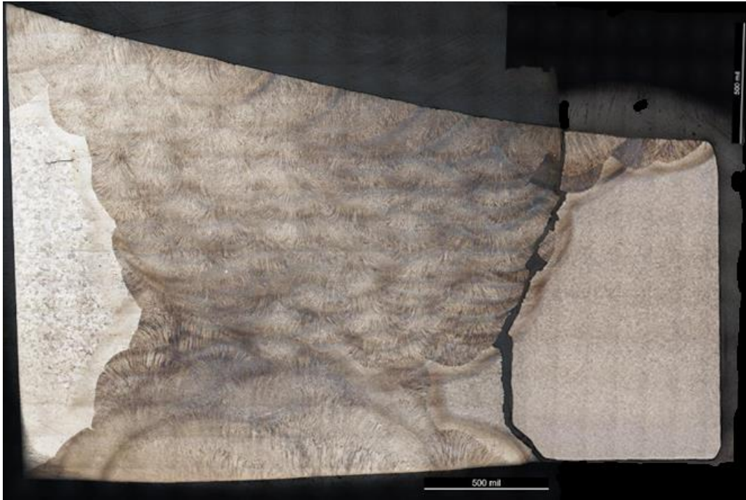
Figure 36. Primary (lower) preexisting crack region shown in a low-magnification montage.
