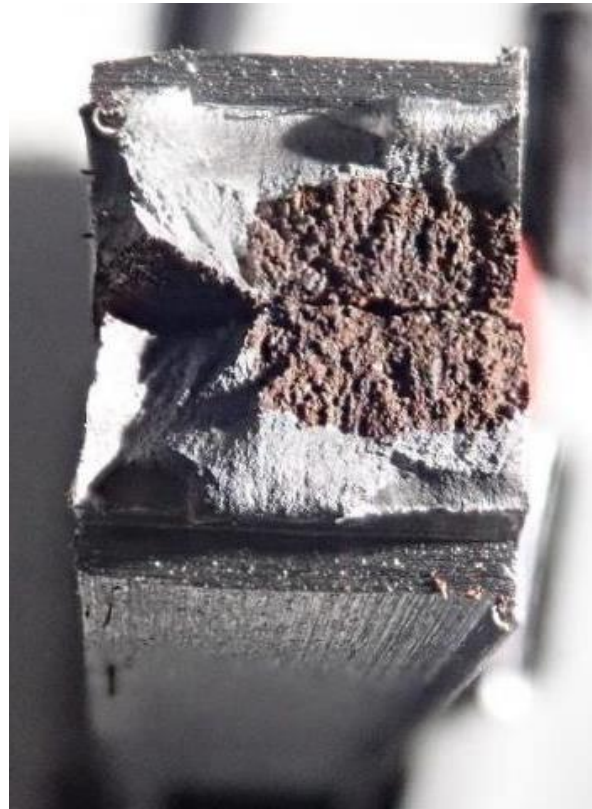
b. Fracture surface of the flaw (circled region from a).
