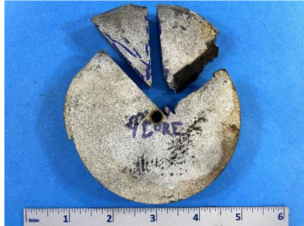
Figure 32. Sectioned core from the arrested crack tip.
