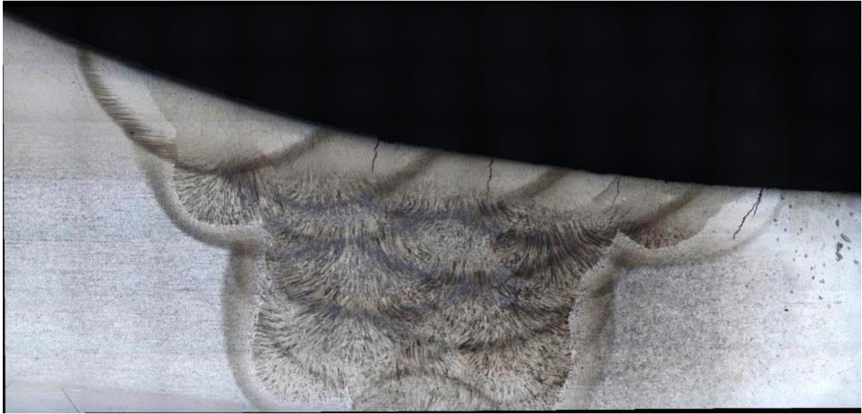
Figure 54. Cracks in the top weld passes at location SA168W
