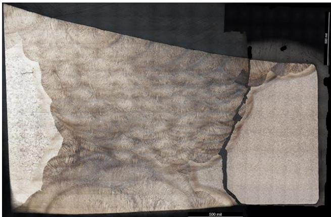
a. Primary Preexisting Crack weld profile.
