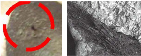
Figure 12. Higher magnification (left) and SEM image (right) of the casting defect shown in figure 9. Proper identification reveals that defect is embedded wire from the paint brush.
