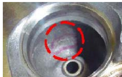
Figure 9. Casting made in permanent mold. Defect detected in the as-cast condition.
