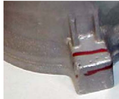
Figure 7. Casting made by using the dry sand process. Defects detected in the as-cast condition.
