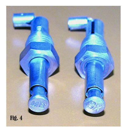
First, note that it has a dull zinc/cad finish and it too has an L-shaped body. But, look closely at the tube surrounding the plunger shaft. It's NOT round like the plunger shaft itself. It has a squared geometry that gives it an interference fit to the OD of the hex installation nut.
