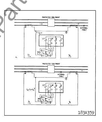
Fig. 3. Schematic Diagrams of the Type CA-5 Relay. (A) Shows the Fault Current Distribution for an External Fault; (B) The Distribution for an Internal Fault.
