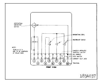
Fig. 1. Internal Schematic of the Type CA-5 Relay in the Type FT21 case.
