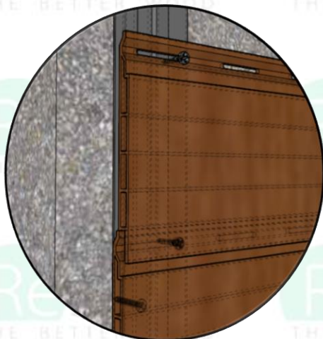
ISOMETRIC DETAIL RESYSTA HORIZONTAL SIDING
