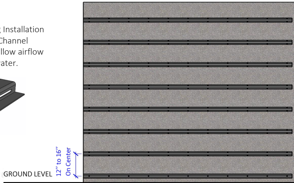
FRONT ELEVATION VERTICAL SIDING / HORIZONTAL BATTENS
