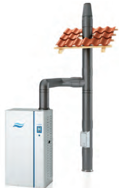
Lower flue gas temperatures allow the use of PVC rather than stainless steel flue
