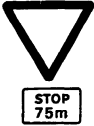
Advance warning of Stop sign.
