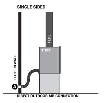
It is preferable to connect to outdoor air in order to optimise combustion control. Depending on specific building-related conditions (air tightness, presence of mechanically controlled ventilation, presence of a kitchen hood, etc).
