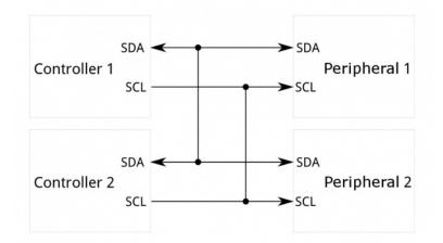
$I^2C$  requires a mere two wires, like asynchronous serial, but those two wires can support up to 1008 peripheral devices. Also, unlike SPI, AC can support a multicontroller system, allowing more than one controller <sup>[11]</sup> to communicate with all peripheral <sup>[11]</sup> devices on the bus (although the controller devices can't talk to each other over the bus and must take turns using the bus lines).
