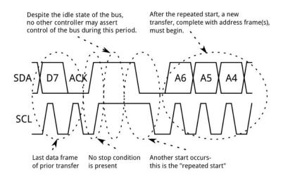
To perform a repeated start, SDA is allowed to go high while SCL is low, SCL is allowed to go high, and then SDA is brought low again while SCL is high. Because there was no stop condition on the bus, the previous communication wasn't truly completed and the current controller maintains control of the bus.
