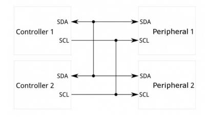
The Inter-Integrated Circuit (I<sup>2</sup>C) Protocol is a protocol intended to allow multiple "peripheral" digital integrated circuits ("chips") to communicate with one or more "controller" chips. Like the Serial Peripheral Interface (SPI), it is only intended for short distance communications within a single device. Like Asynchronous Serial Interfaces (such as RS-232 or UARTs), it only requires two signal wires to exchange information.
