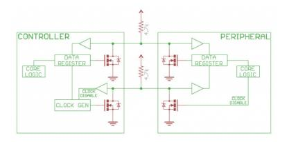
Notice the two pull-up resistors on the two communication lines.
