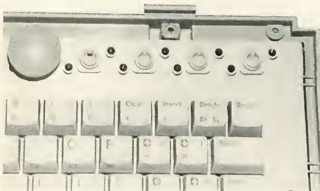
There's room at the top of this keyboard for the START, SELECT, OPTION and RESET keys. But they are in the console. A dead giveaway that this keyboard is identical to that of the 65XE.
