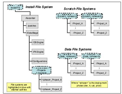
Figure 4-4 Suggested DataStage installation, projects, data, and scratch file systems
