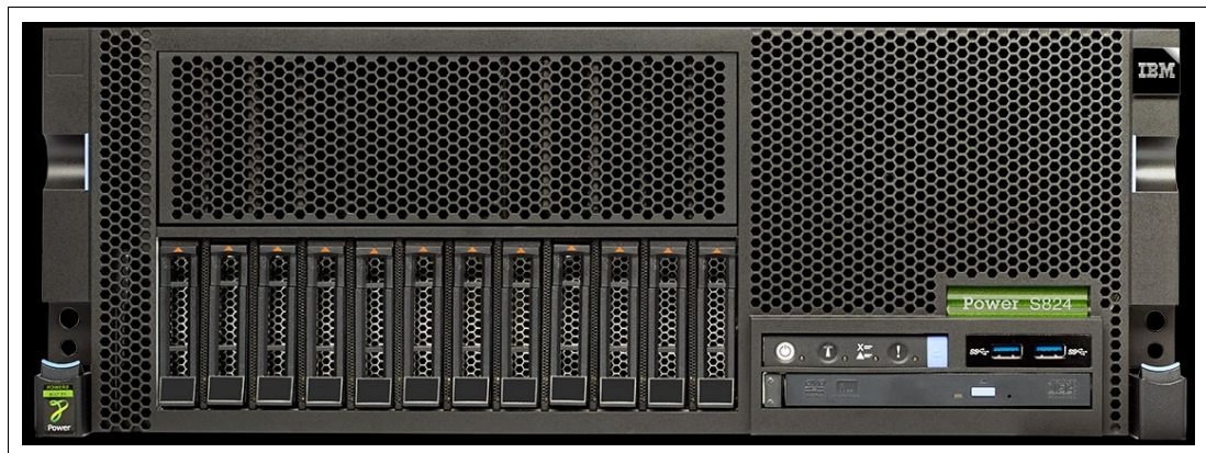
Figure 1-5 Front view of the Power S824 system
