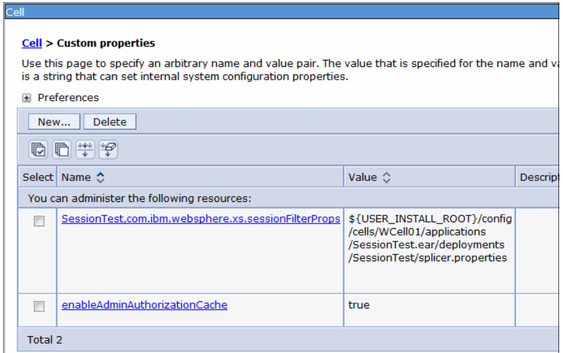
Figure 6-20 A new cell-scoped custom property that provides the location of the splicer.properties
