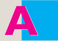
Without Trapping when misregistration on the Press
