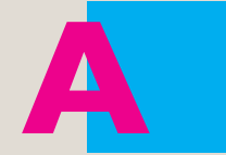
With Trapping when misregistration on the Press
