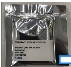
Figure 2. ICELL8 3' DE Chip Packaging. The chip is sealed along with a silica packet. Be careful not to cut the silica packet when opening the pouch.
