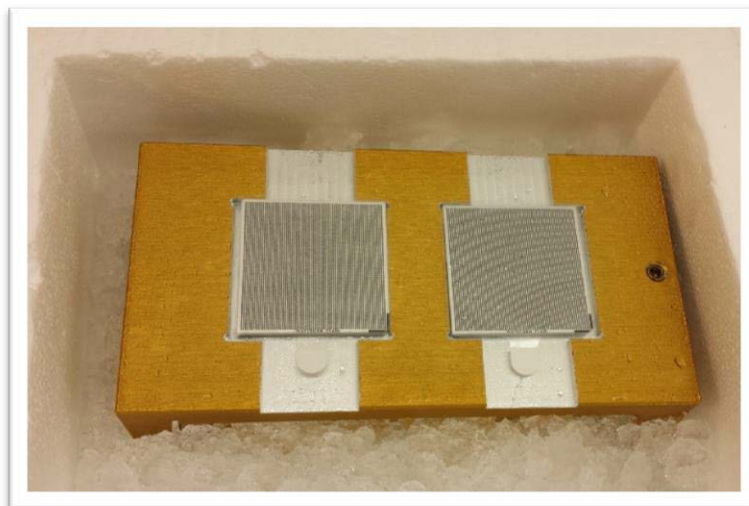
Figure 37. Place the chip on a cold block on ice.
