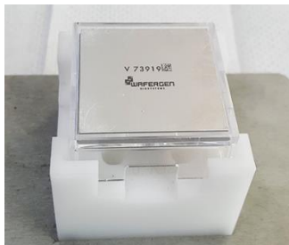
Figure 42. Place chip into Collection Module
