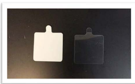
Figure 12. TE Sealing Film (white background) and Optical Imaging Film (transparent background). The Imaging Film has three layers; the intermediate layer is double-sided.
