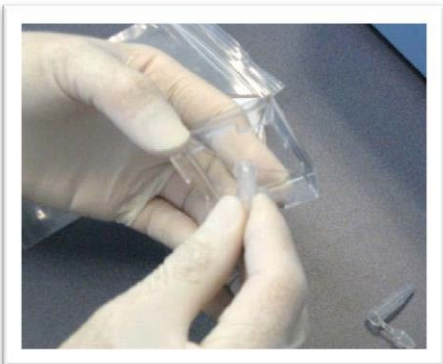
Figure 40. Attach the Collection Tube to a Collection Fixture.
