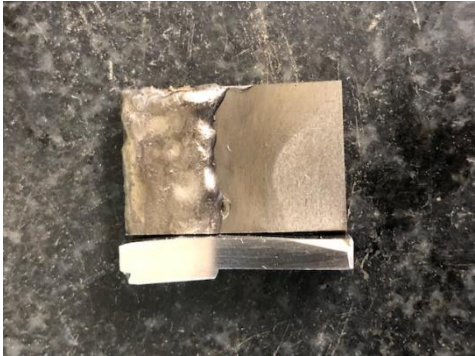
Haynes 282 sheet with 224 weld overlay in place
