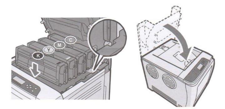
Reinstall the cartridges in the desired configuration (in the above representation, white or black can go into the first slot) and close the lid. Use white for transfer printing and black for normal CMYK printing.
