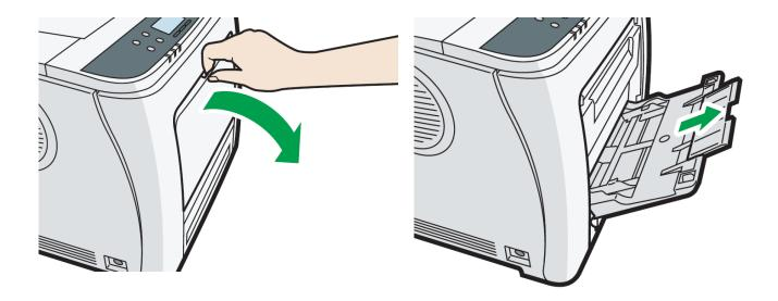
To access the MPT tray, press and hold the lever at the top and pull out and down. Pull out the extender when loading paper larger than A4 or letter size.
