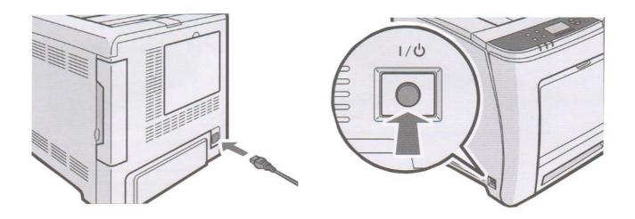
Insert power cord and power on the unit as per the driver installation instructions. If connecting via USB, do not plug in the USB cable until instructed to do so by the software.
