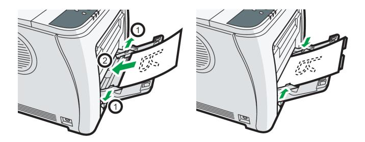
Load the paper print side face down and adjust the guides as necessary.
