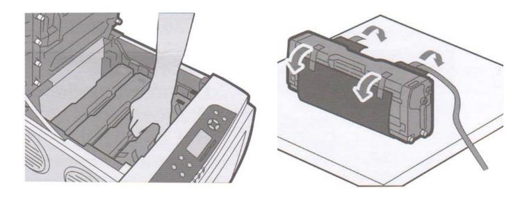
Remove the white toner cartridge from the front of the machine. Place it on a flat, solid surface and carefully remove the black security paper.
