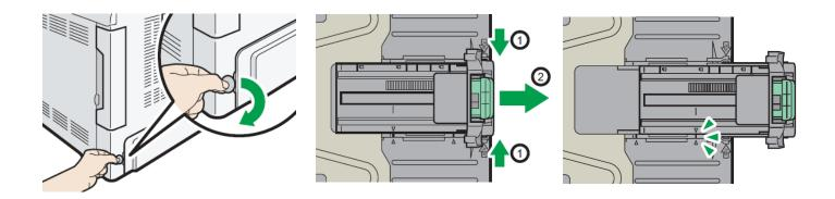
When loading paper longer than 11" into tray 1, remove the lower rear cover using a coin. Squeeze the rear extender and push outward to accommodate lengths up to 14" long. Do not extend this tray when loading A4 or letter size paper. Otherwise, a paper jam may occur.
