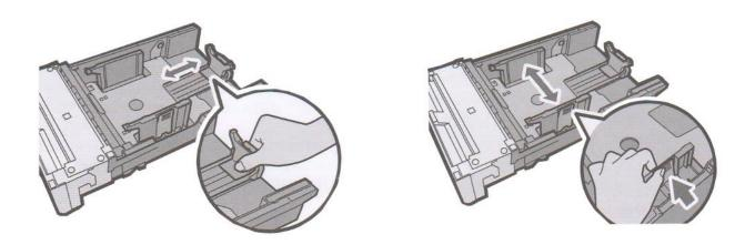
Squeeze the clips on the paper guides and slide them to match paper size. Do not move the paper guides forcefully. Doing so may damage the tray.
