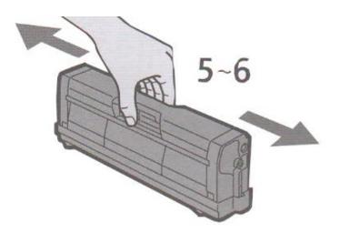
Remove each cartridge and gently shake back and forth 5 or 6 times to loosen the toner that may be settled in the cartridge due to shipping.
