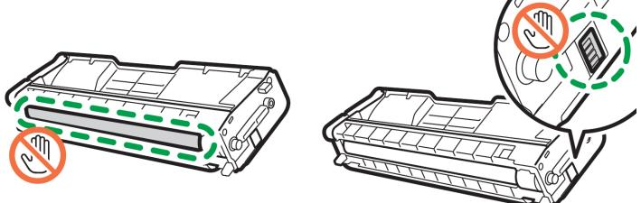
• When removing print cartridges, be careful not to touch the laser scanning unit under the upper cover (the position shown by the arrow in the illustration to the right).
