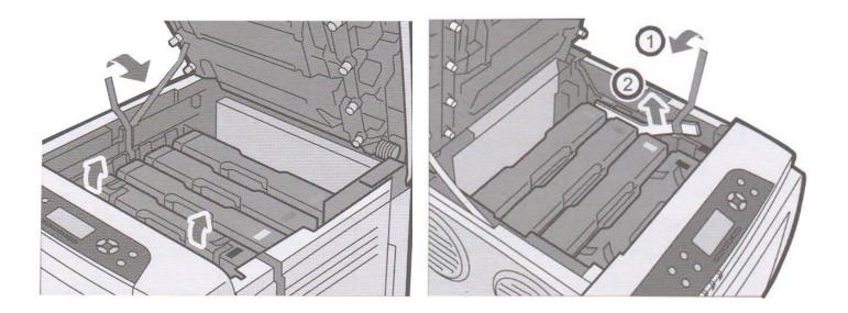
Remove orange security tape and packing material from inside the printer.
