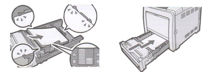
Load media with the print side face up and ensure it locks in underneath the guides before closing the cassette. Ensure the paper stack does not exceed the upper limit mark inside the paper tray. Excess stacking can cause paper jams.
