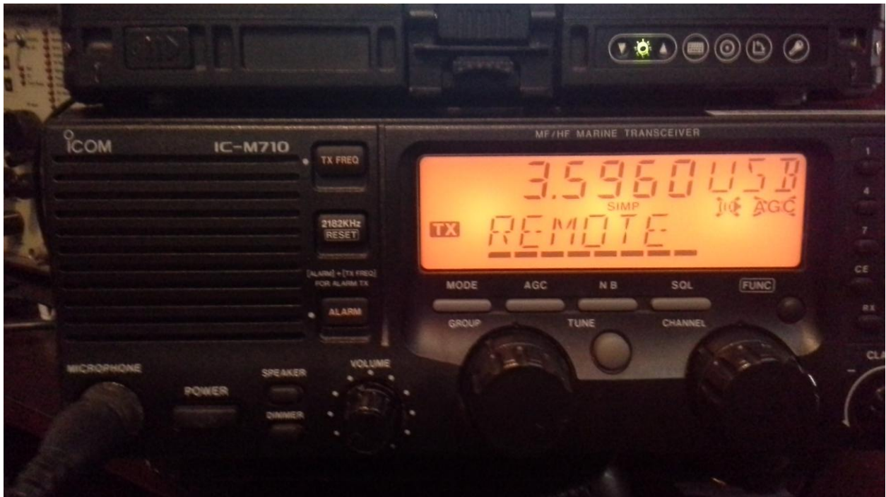
Here is the M710 using the custom MMI files, in Transmit, USB mode.
