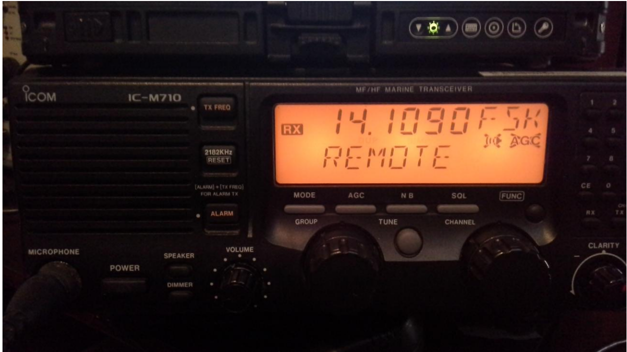
Here is the M710 using the custom MMI files in FSK mode in receive using the 6 kHz filters. Mute is ON, AGC is OFF, NB is OFF, SQL is OFF. High power selected.
