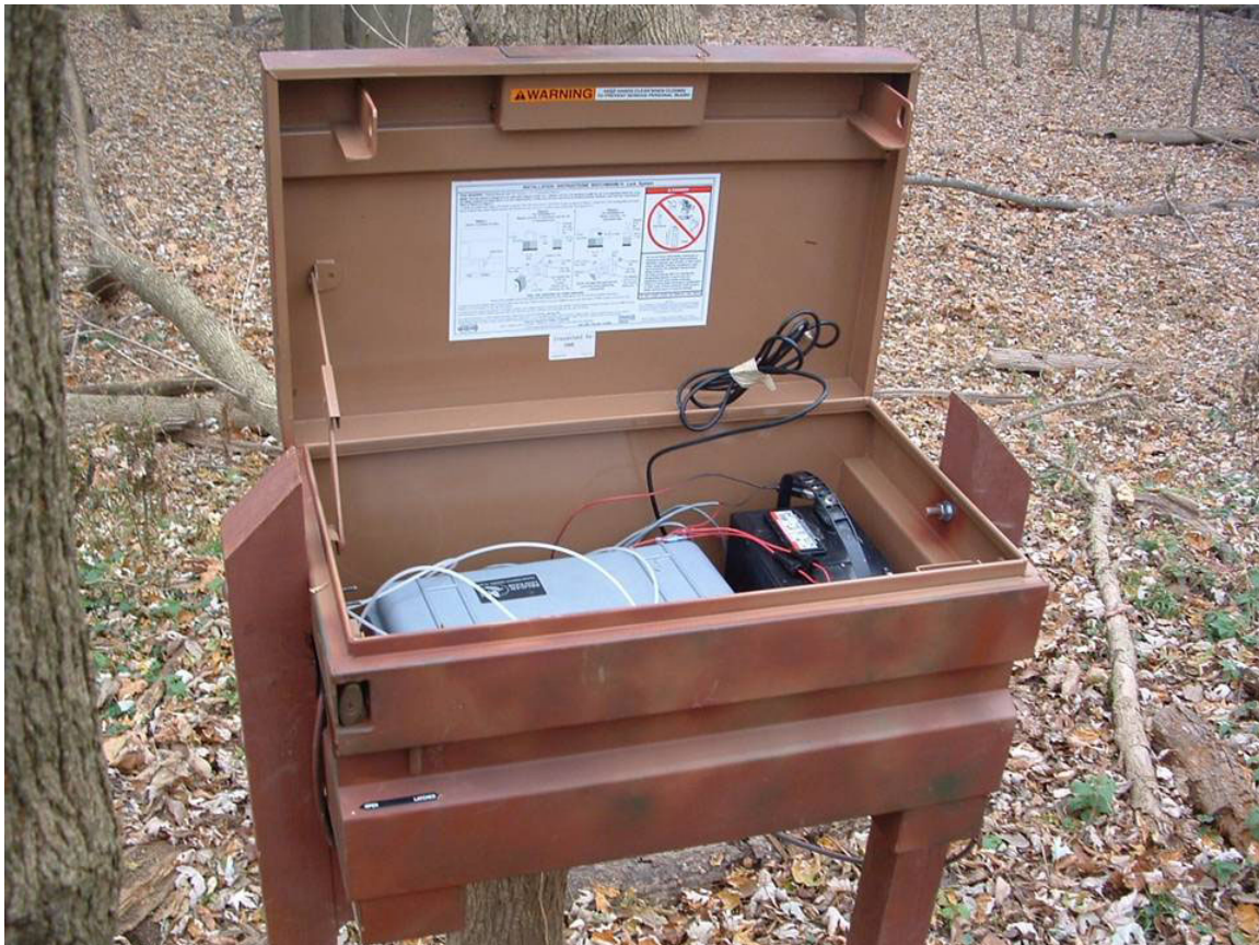
Figure 1: Inside the river level monitor at Edwards Ferry
