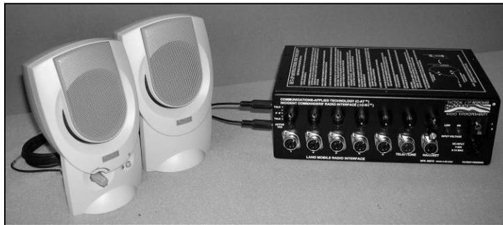
**FIGURE 24: ICRI SPEAKER CABLE CONNECTED TO SPEAKER JACKS**
