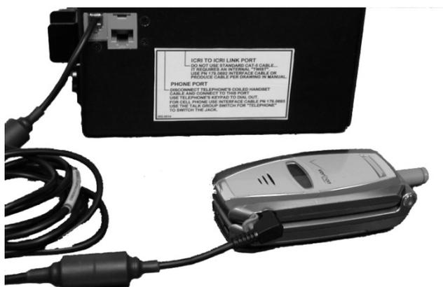
**FIGURE 20: ICRI CONNECTED TO CELLULAR PHONE THROUGH RJ22**
