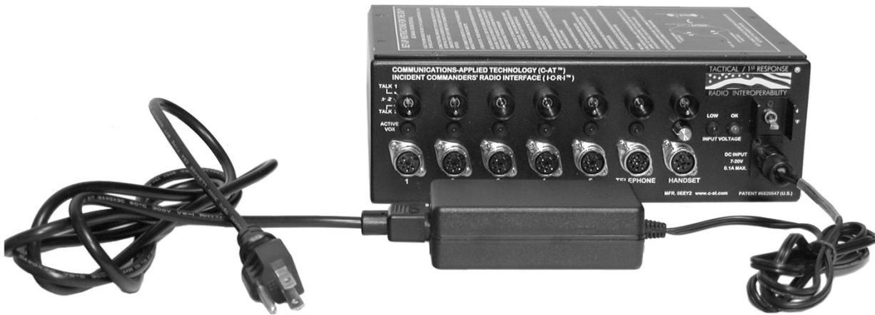
**FIGURE 10: ICRI WITH EXTERNAL POWER SUPPLY**
