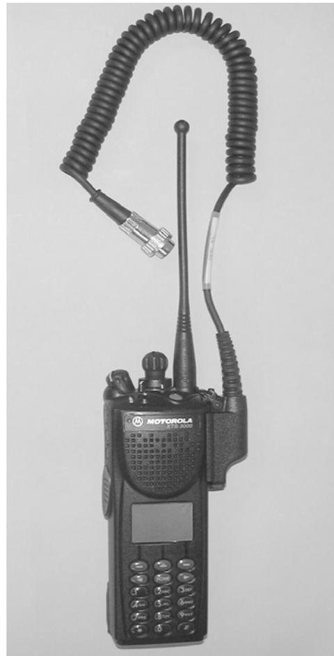
**FIGURE 13: RADIO WITH ICRI INTERFACE CABLE**
