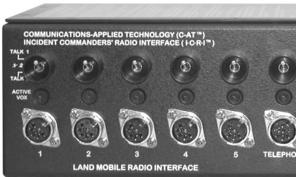
**FIGURE 12: ICRI INTERFACE JACKS AND TALK GROUP SELECTOR SWITCHES**
