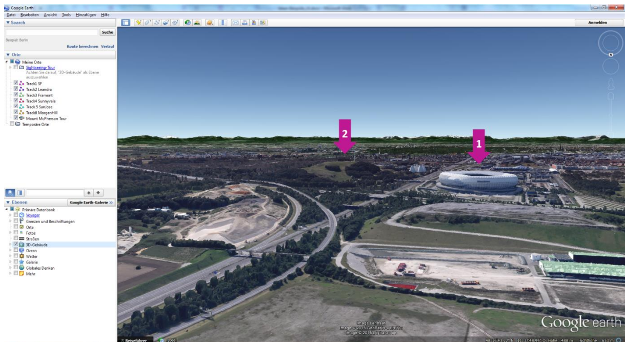
Fig. 10: Two possible positions for a small PV solar power plant, visualized in Google Earth 12 : (1) on the roof of a football stadium, (2) on the top of a small hill close by.
