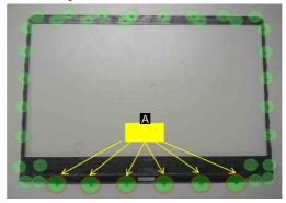
Adhesive tape on the back side of LCD front bezel
