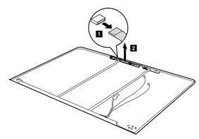
When installing: Stick the integrated camera to the top center of the LCD cover and adjust the placement of it to make sure the connector is attached firmly.
