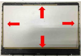
Figure 10. Removal steps of LCD front bezel (continued)
