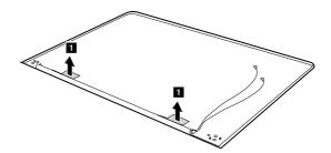
When installing: Route the antenna cables along the cable guides and secure the antenna boards with adhesive tapes. As you route the cables, make sure that they are not subjected to any tension. Tension could cause the cables to be damaged by the cable guides, or a wire to be broken.
