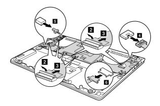
When installing: Make sure that all the connectors are attached firmly
