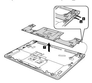
When installing: When attaching the system board to the base cover, adjust the placement of the USB, AC power adapter ports as shown in a, b, and make sure that they are attached to the holes on the base cover as shown. Improper placement of those jacks might cause a damage.
