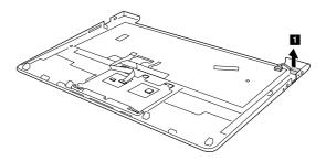
Remove screws , and then remove the touchpad module in the direction shown by arrow 2.
