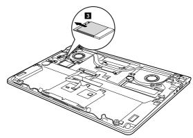
In step , unplug the jacks by using the removal tool antenna RF connector (P/N: 08K7159), or pick up the connectors with your fingers and gently unplug them in the direction shown by the arrows.
