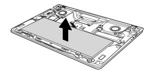
When installing: Make sure that the battery connector is attached firmly.
