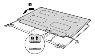
When installing: Make sure that the connector is attached firmly.
