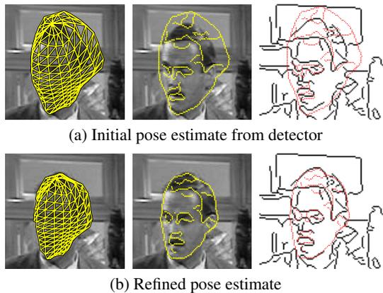
**Figure 6. Pose refinement.** The initial pose estimate (a) from the detector tree is refined by chamfer matching to give the final estimate (b). Columns show respectively the head model, rendered edges overlaid on the input image, and rendered edges overlaid on the edge image.
