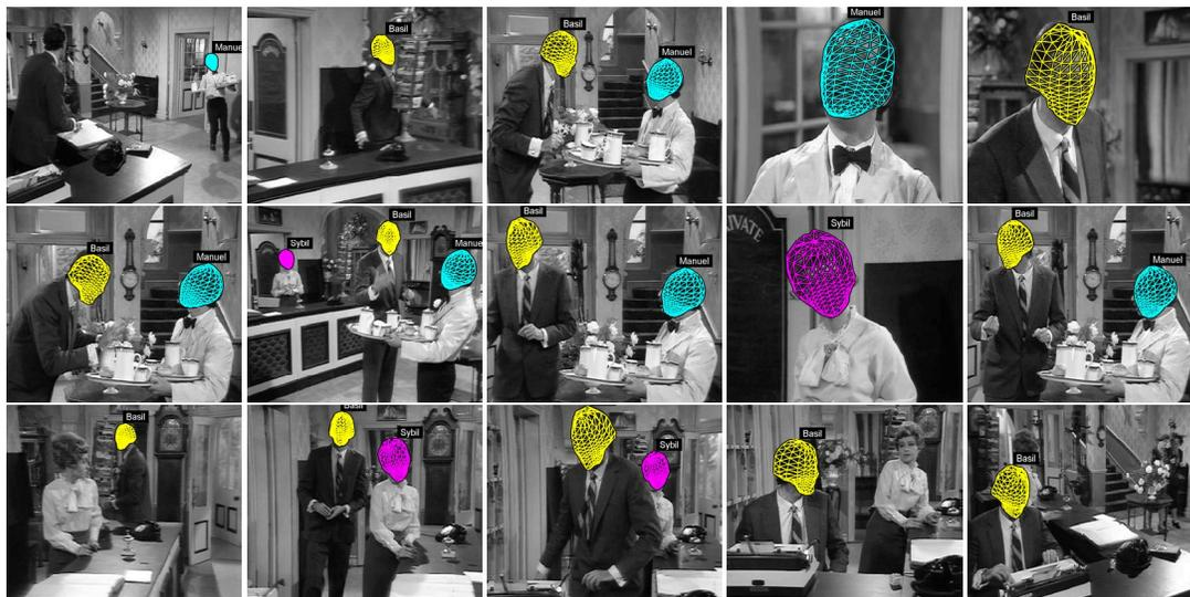
**Figure 7. Example detections and identifications. Frames from a video sequence of 15 shots of ‘Fawlty Towers’ are shown with the head model of the identified character overlaid in the estimated pose. The three main characters are detected and identified over a wide range of scale and pose.**
