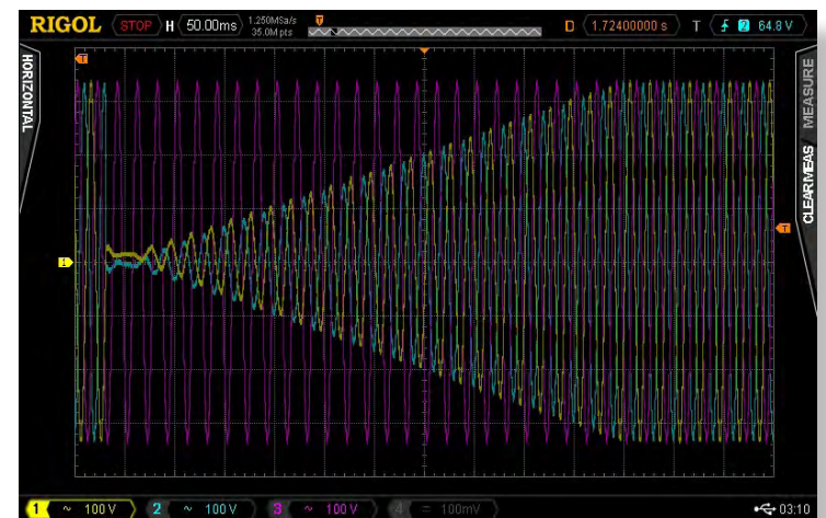
Figure 17: IEC 61000-4-34 Three Phase Voltage Variation Test
