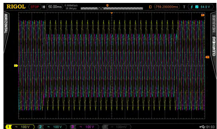
Figure 5: IEC 61000-4-11 Phase BC Voltage Dip to 70% of UT
