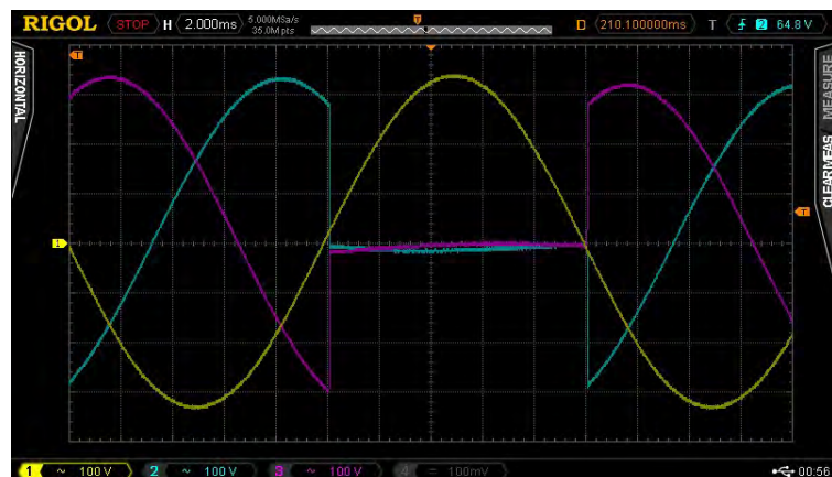
Figure 4: IEC 61000-4-11 1/2 Cycle Phase-to-Phase Voltage Dip
