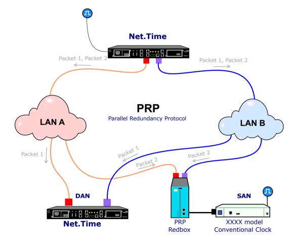
PRP is based on the use of two independent networks. The sender **must send each packet twice** (to LAN A and LAN B) through two separate ports. There are two types of devices:
