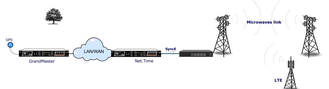
Net.Time supports Synchronous Ethernet over a copper and optical connections. This allows operators to utilize cables on SFP ports and still meet timing and synchronization requirements for demanding applications like LTE in mobile networks and microwaves links.
