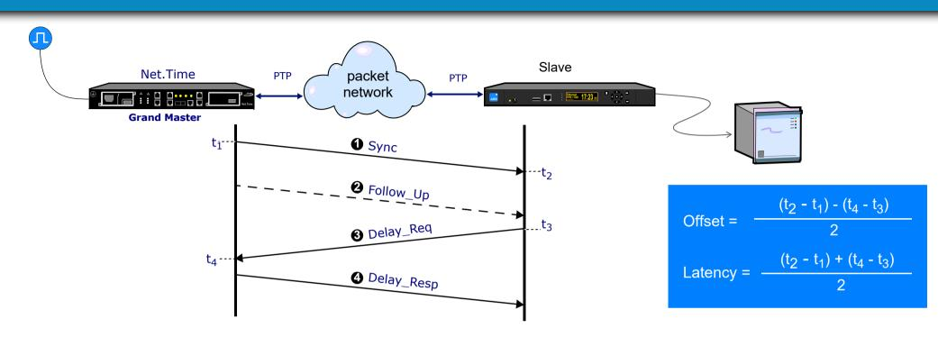
It is a cost-efficient solution and can be applied on the basis of the existing Ethernet network in a substation. PTP (IEEE 1588) applies master/slave time synchronization mechanisms and supports hardware time stamps. The basic parameters of Latency / Offset are computed from the  $t_{1...4}$  stamps.
