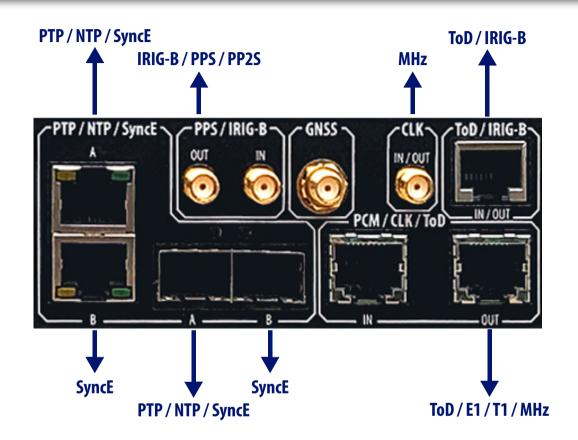
Can be defined the sequence of alternatives in case of the main time reference failure.
