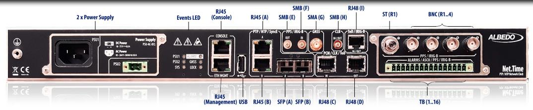
Net.Time is a boundary clock designed to simplify migration to PTP protocol from previous generation architectures. Net.Time offers seamless translation while offering a high variety of clock reference inputs and outputs that may be used as primary or backup references, monitoring and synchronization.
