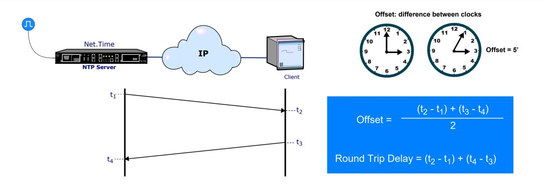
NTP can provide a milisecs range of precision which is good enough for most of enterprise applications.
