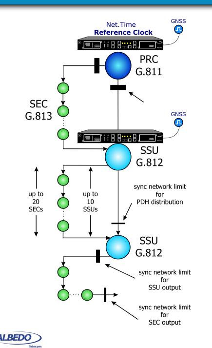
Net.Time configured as PRC is equipped with Rubidium oscillator providing timing to the SSU that can be a Net.Time with OCXO oscillator.
