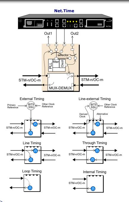
In SDH/SONET there are four ways to synchronize ADM and digital cross connects (DXC):
