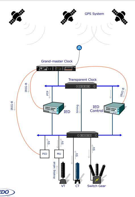
Many Utilities acquire timing from GNSS and the station clock converts signal into a 1-pps or IRIG-B code, which are then distributed by dedicated links to all the IEDs in a substation. However, important to say that this system has some **weaknesses** (\*) being **vulnerable** to human and natural disruptions that may perturb normal operations by raising false alarms, delaying actions, and lowering system efficiency.
