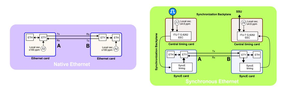
SyncE is not part of the IEC 61850 but is being used in the Power industry
