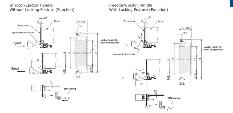
Injector/Ejector Offset Handle With Locking Feature (Function)
