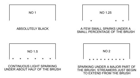
NOTE—Each diagram represents the trailing edge of one brush. If brushes are different, record condition of each, identifying them 1, 2, 3, etc., from riser end. (See NEMA CB 1-1995.) For the degrees of sparking involved here, spitting, glowing spots, and leading edge sparking are not normal.
